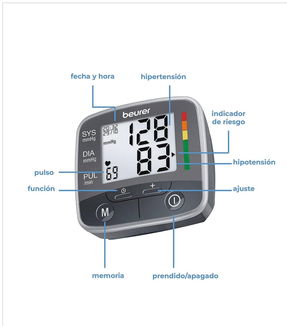
Image 3: Diagram illustrating the various parts of the Beurer BC32 monitor, including the display for date, time, hypertension/hypotension indicators, pulse, function, memory, and power buttons.
