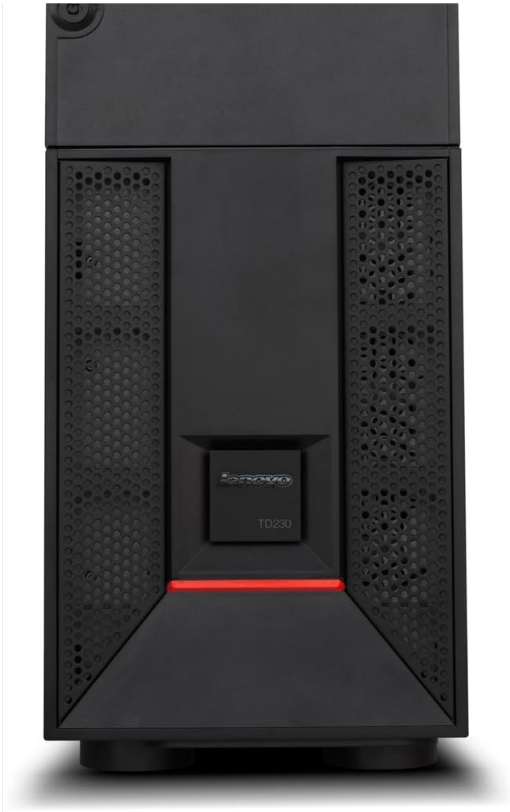
Figure 2.2: Front view of the Lenovo Thinkserver TD230 tower server. This image provides a clear look at the front panel, including the power button, status indicators, and the Lenovo TD230 branding.
