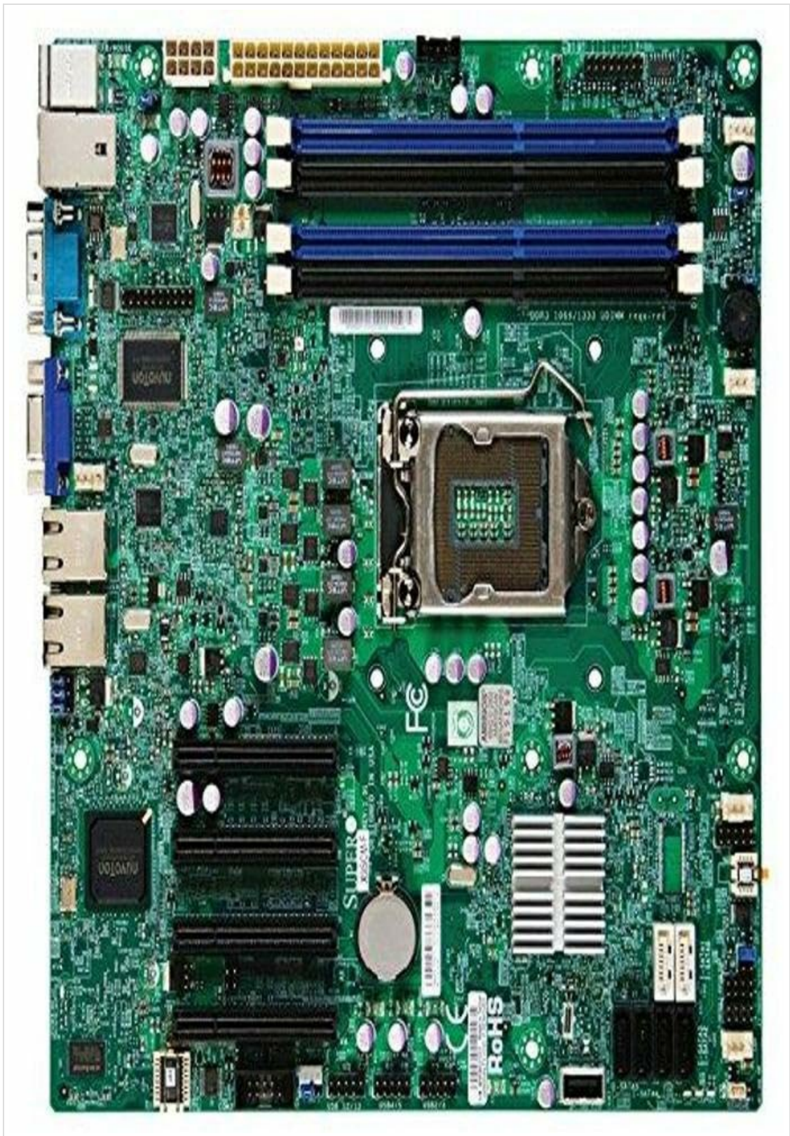
Image: Supermicro MBD-X9SCM-F-O Server Motherboard. This image displays the top-down view of the motherboard, highlighting the CPU socket, DIMM slots, PCI-Express slots, and various connectors.
