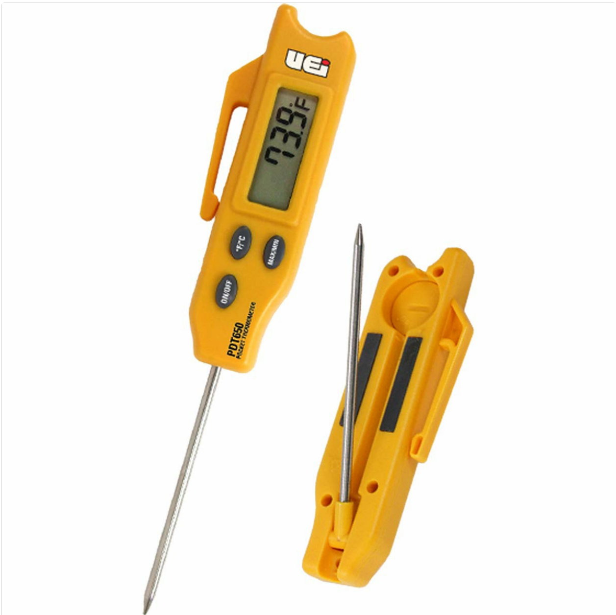
Image: A close-up view of the UEi PDT650 thermometer with its probe extended, clearly showing the digital display, ON/OFF, °F/°C, and MAX/MIN buttons.
