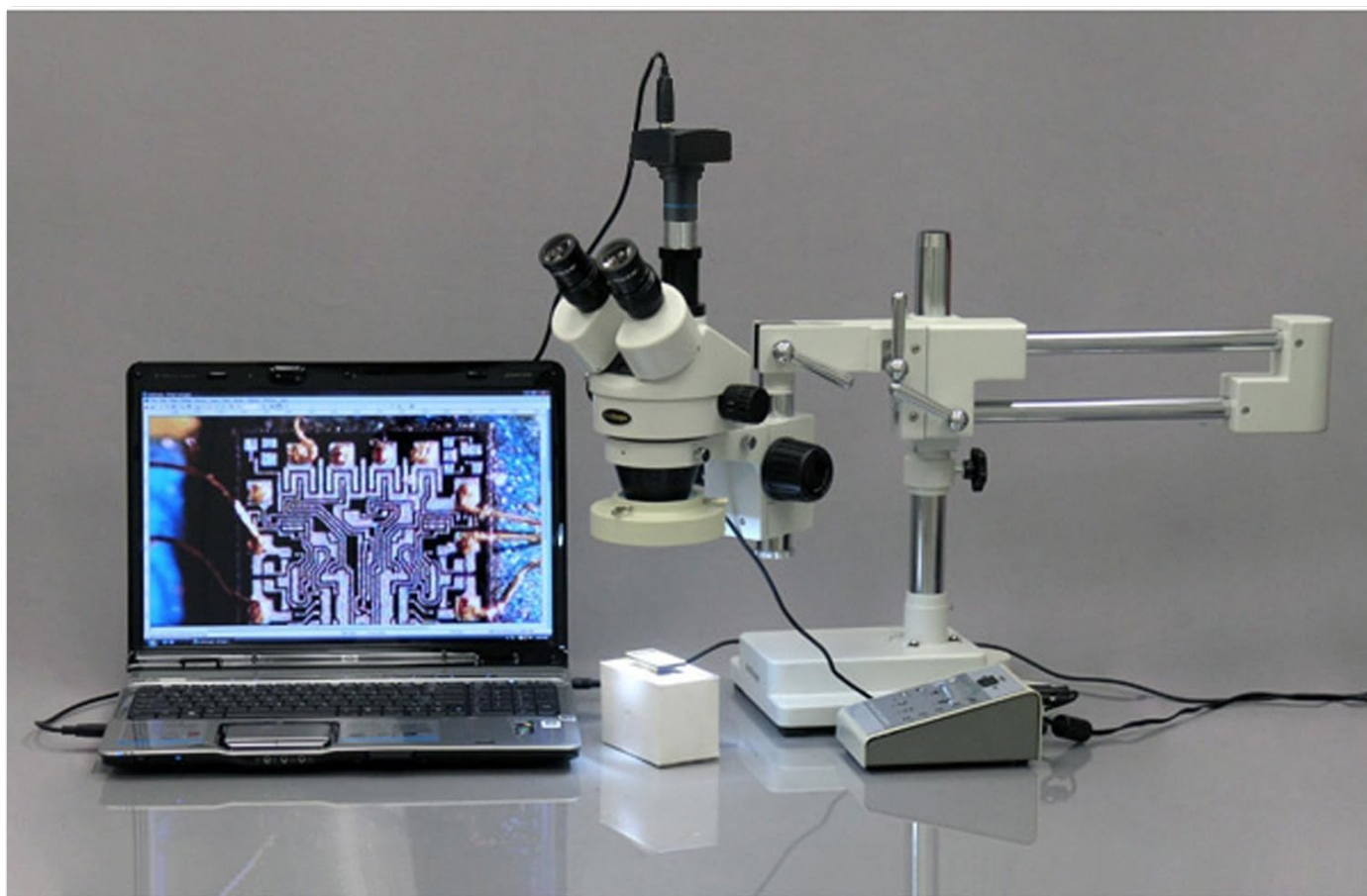
Image: The AmScope MU800 camera mounted on a stereo microscope, connected via USB to a laptop displaying the live microscope feed.
