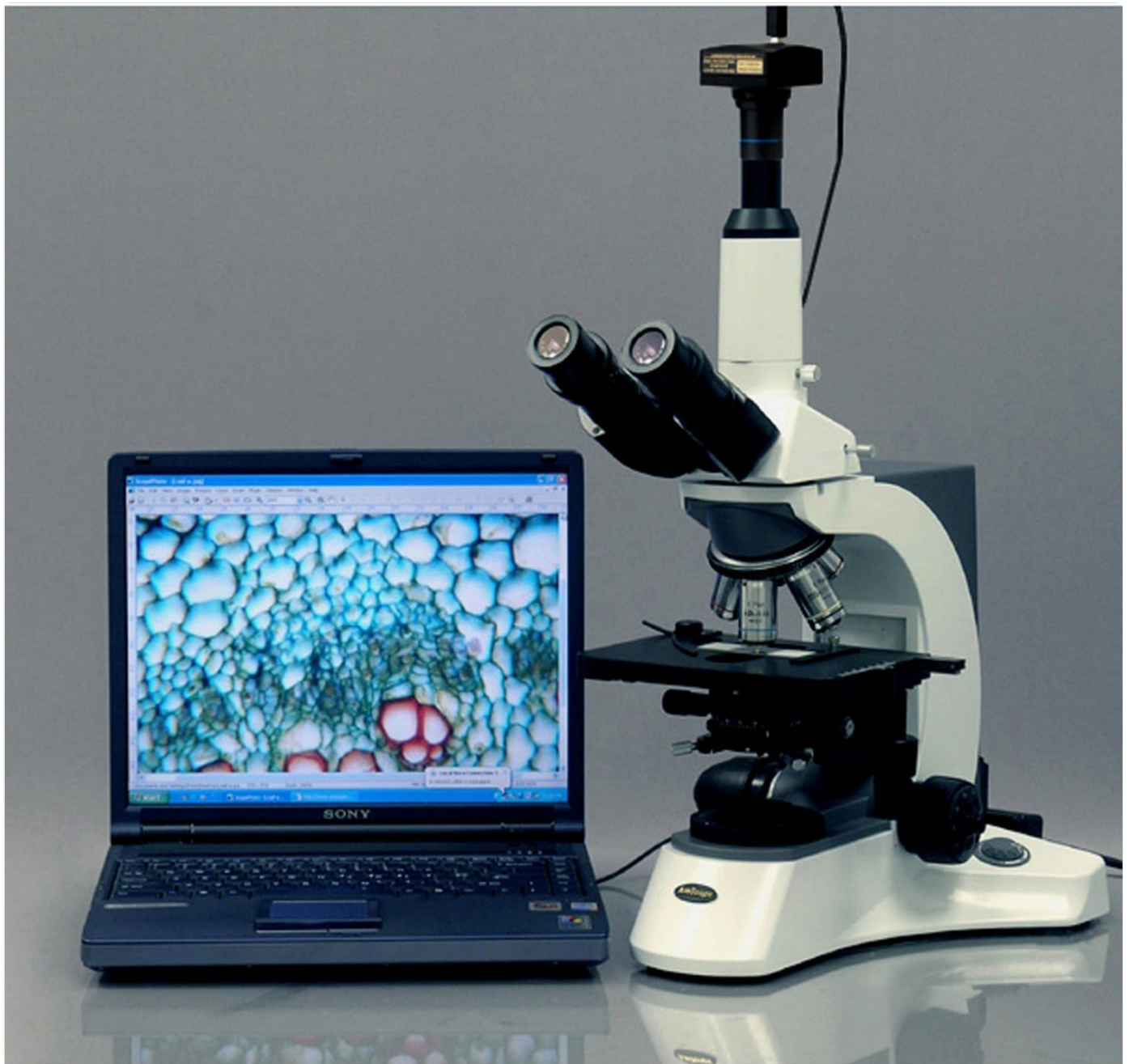
Image: The AmScope MU800 camera mounted on a compound microscope, connected via USB to a laptop displaying the live microscope feed.
