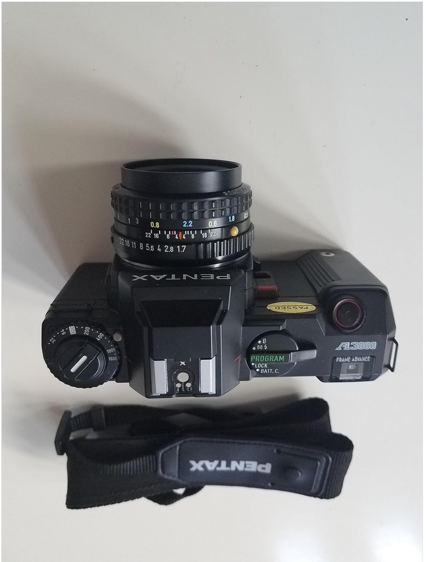
Figure 3.2: Detailed view of the camera lens, highlighting the aperture ring, focus ring, and depth of field scale. The Pentax brand name is visible on the camera body.
