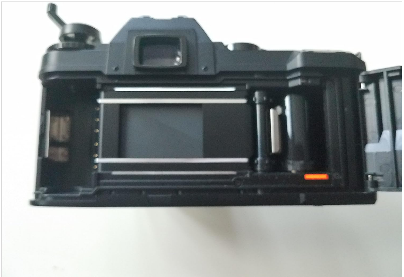
Figure 4.1: Rear view of the Pentax A-3000 with the film compartment open, illustrating the film chamber on the left and the take-up spool on the right.
