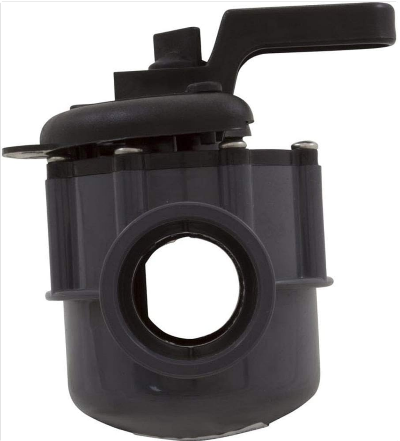
Figure 3.4: End view of the valve, showing one of the 1-1/2 inch connection ports. This port is designed for solvent welding to standard PVC or CPVC piping.
