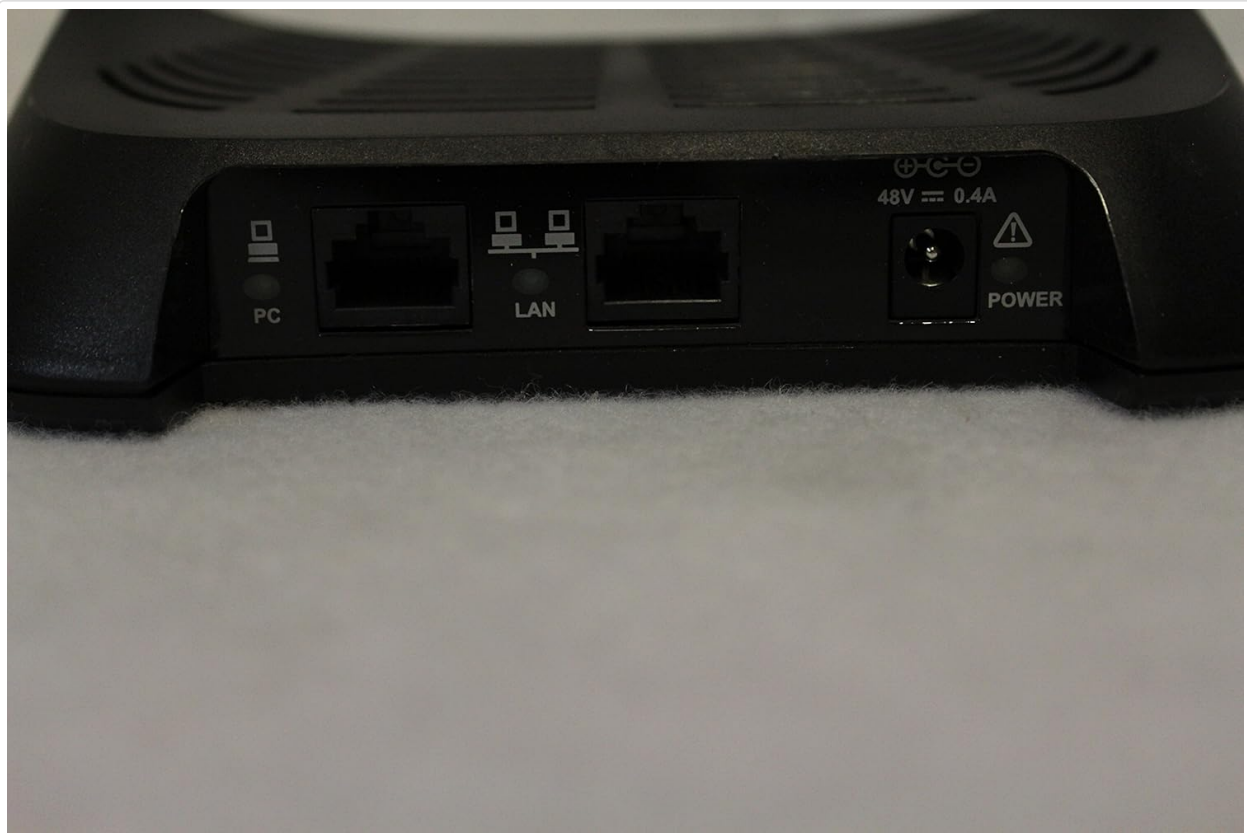
Figure 2: Rear view of the Mitel Gigabit Ethernet Stand, highlighting the PC, LAN, and Power input ports. The power input specifies 48V === 0.4A.
