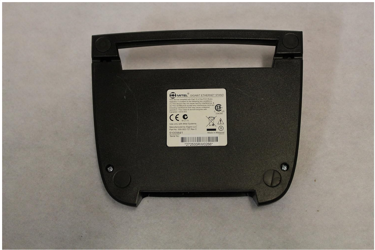
Figure 5: Underside of the Mitel Gigabit Ethernet Stand, illustrating the structural design, screw points, and rubber feet for stability.
