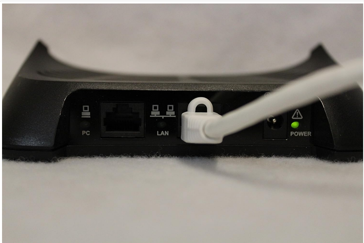
Figure 3: Rear view of the Mitel Gigabit Ethernet Stand with a white Ethernet cable connected to the LAN port, demonstrating a typical setup. A green power indicator light is visible.
