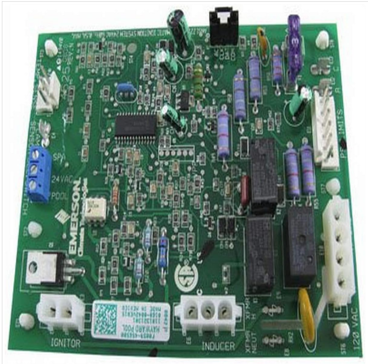
Figure 1: Hayward IDXL2ICB1931 Integrated Control Board. This image displays the green circuit board with various electronic components, including capacitors, resistors, relays, and integrated circuits. Key connection points are labeled, such as "IGNITOR," "INDUCER," "24VAC," "POOL," and "120 VAC."
