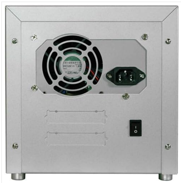
Figure 3.4: Rear View. This image shows the back panel of the RipBox, featuring the power input, cooling fan, and the main power switch.
