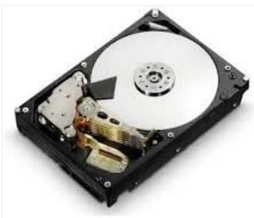
An internal view of the hard drive, showing the platters and read/write heads. This image illustrates the internal components of a typical 3.5-inch mechanical hard disk drive.
