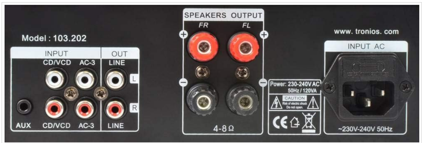
Figure 4.2: Rear view of the Skytronic 103.202 amplifier, showing input/output connections and power inlet.
