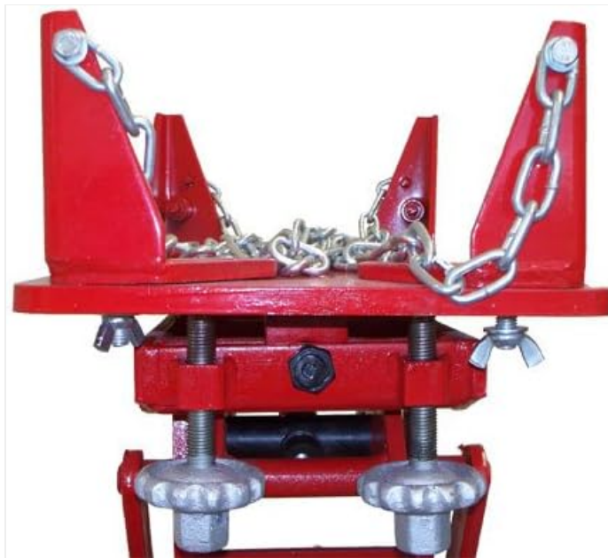
Figure 5.3: Top view of the saddle with chains for securing the load.
