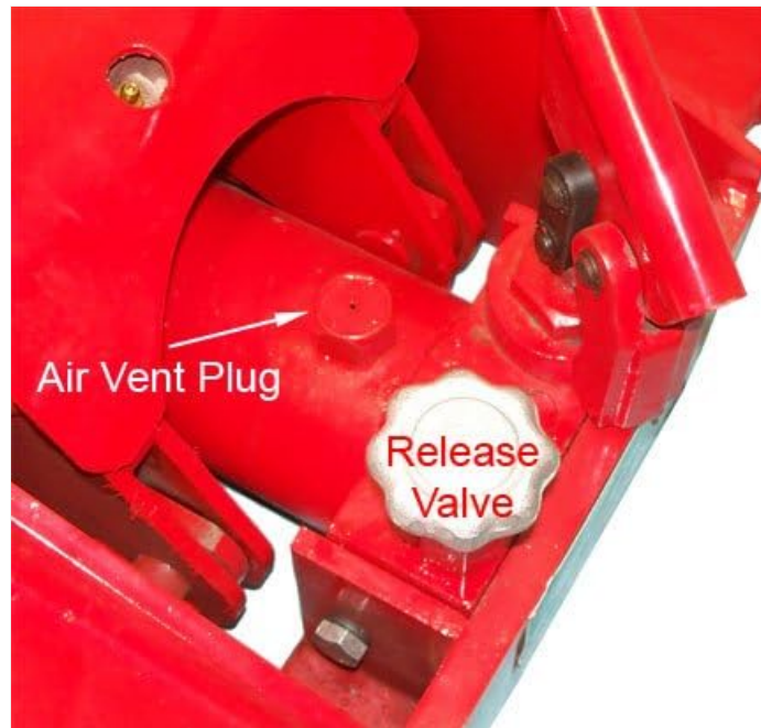
Figure 3.3: Location of the Air Vent Plug and Release Valve on the hydraulic unit.
