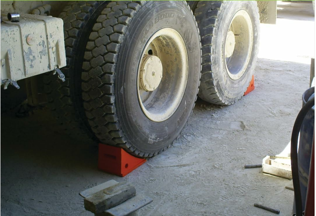
Image 3.1: Two Checkers UC chocks securing the rear wheels of a truck. These chocks are designed to resist weather, fuel, and oils, and will not crack, rot, or splinter like wood or rubber chocks. Their lighter weight compared to traditional chocks makes them easier to maneuver.
