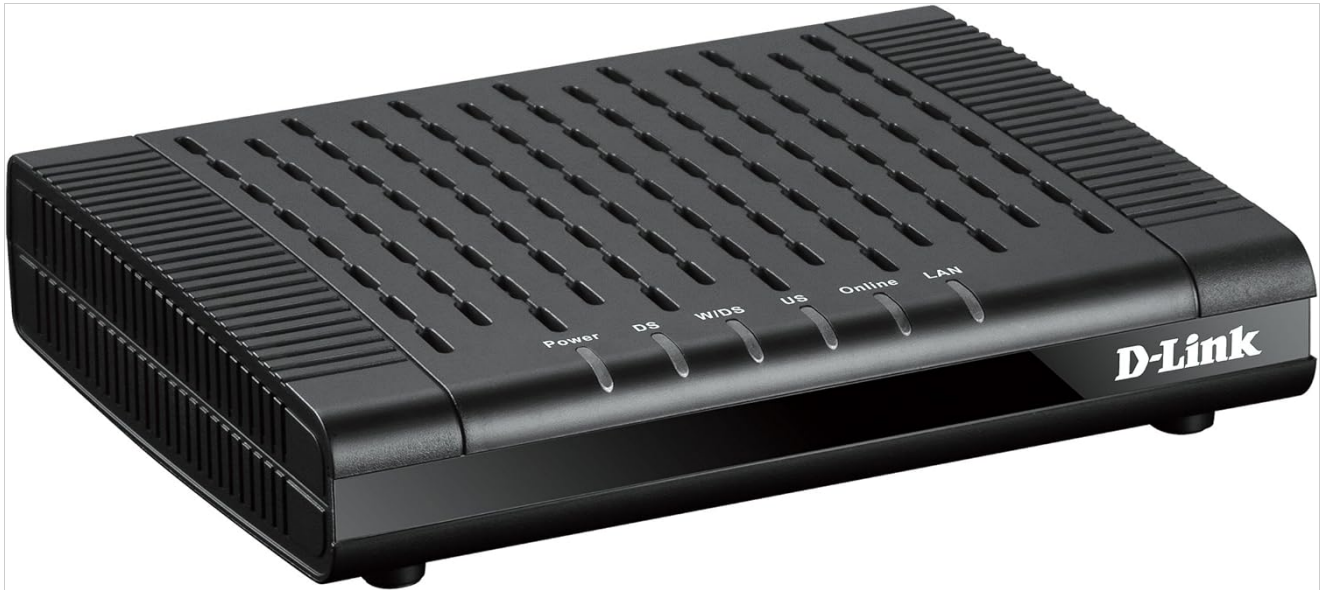
Image: Front view of the D-Link DCM-301 Cable Modem, showing the LED indicators for Power, DS (Downstream), WIDS (Wideband Downstream), US (Upstream), Online, and LAN. These lights indicate the modem's operational status.
