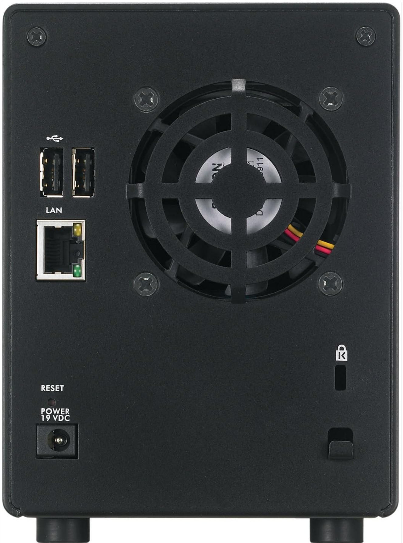
Figure 3.2: Rear view of the ZyXel NSA320, showing the LAN port, USB ports, power input, and reset button.
