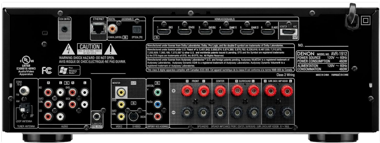
Rear view of the Denon AVR-1912 receiver, highlighting the various input and output ports for audio, video, and network connections.
