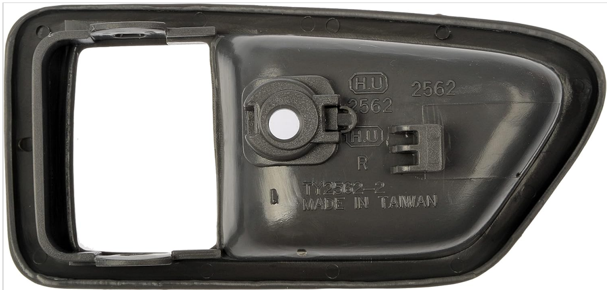
Figure 2: Rear view of the Dorman 91007 Interior Door Handle Bezel, illustrating the mounting points and internal structure for secure attachment.
