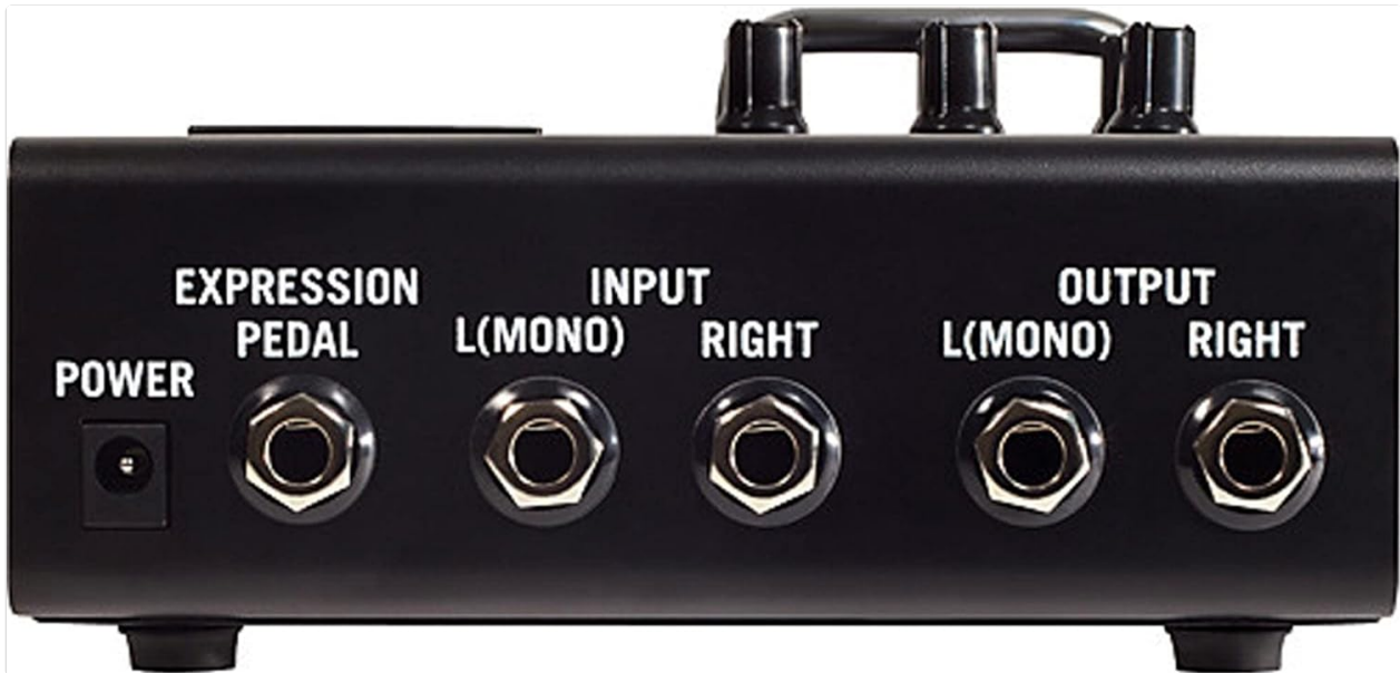
Figure 1: Rear panel connections including power, expression pedal, and audio I/O.
