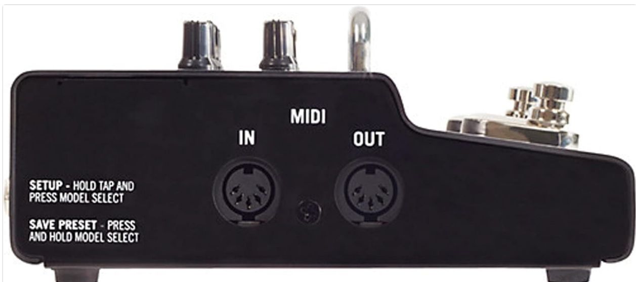
Figure 2: Side panel showing MIDI In and Out ports for external control.
