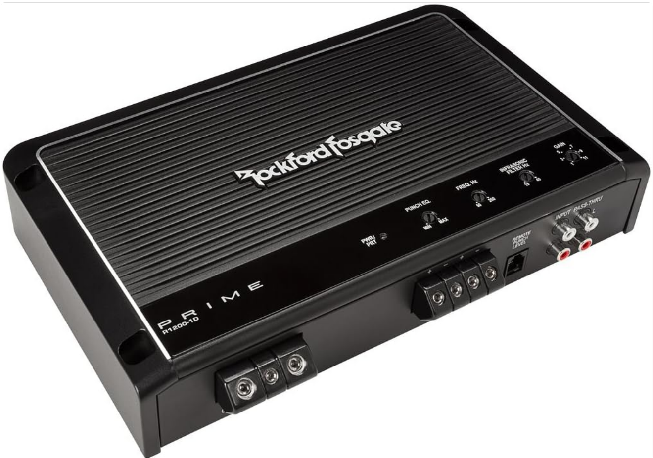
Figure 2: Rear view of the Rockford Fosgate R1200-1D Prime amplifier, detailing the power, ground, remote, speaker, and RCA input/output connections.
