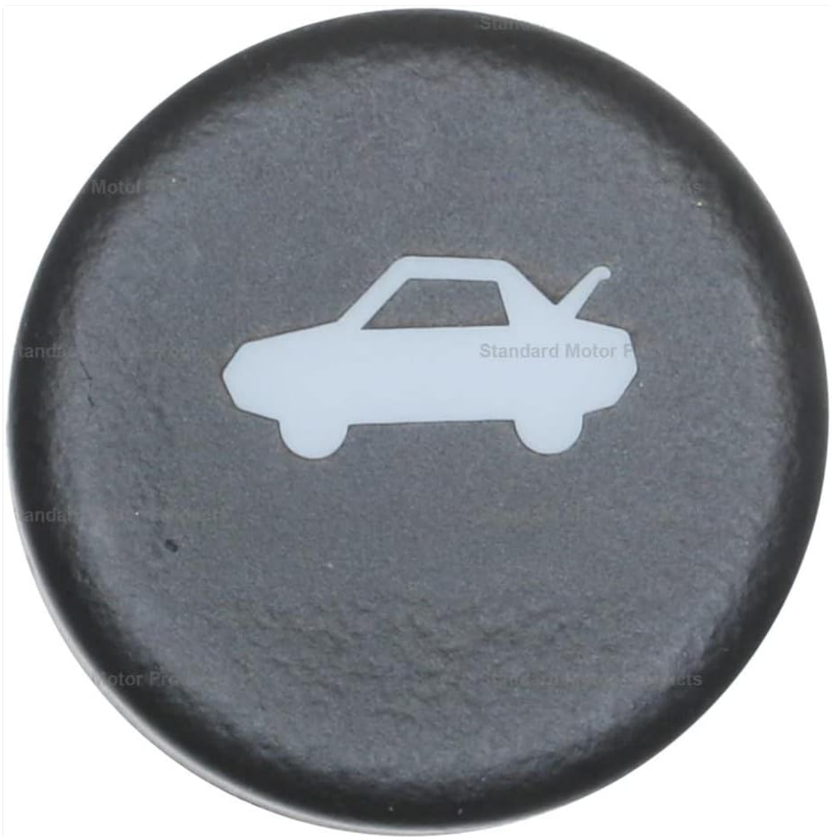
Figure 2: Close-up of the switch button, featuring a white icon depicting a car with an open trunk, indicating its function as a trunk release switch.
