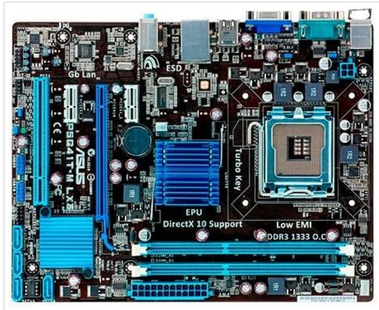
Figure 2.2: Overview of the ASUS P5G41T-M LX3 Motherboard components.
