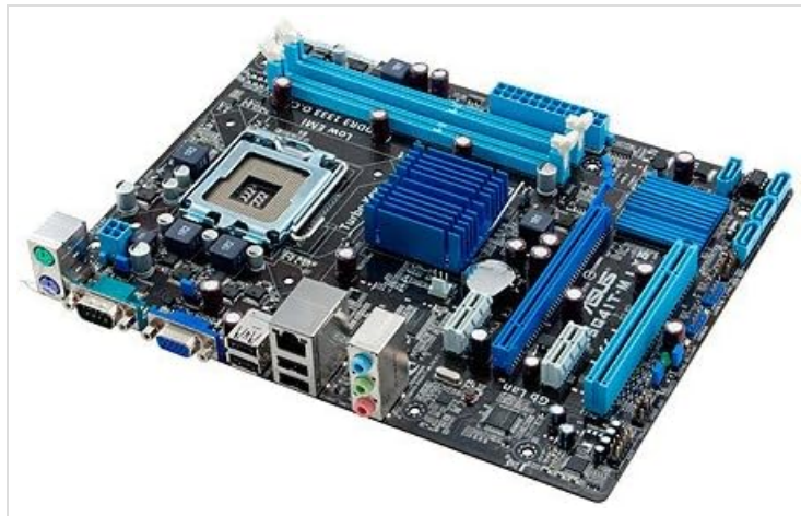
Figure 3.1: Rear I/O panel of the ASUS P5G41T-M LX3 Motherboard.
