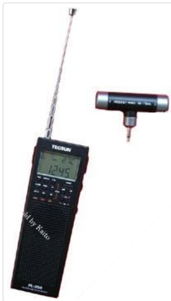
Image 6.1: The Tecsun PL-360 radio with its telescopic antenna fully extended for FM/SW reception, alongside the external AM antenna.
