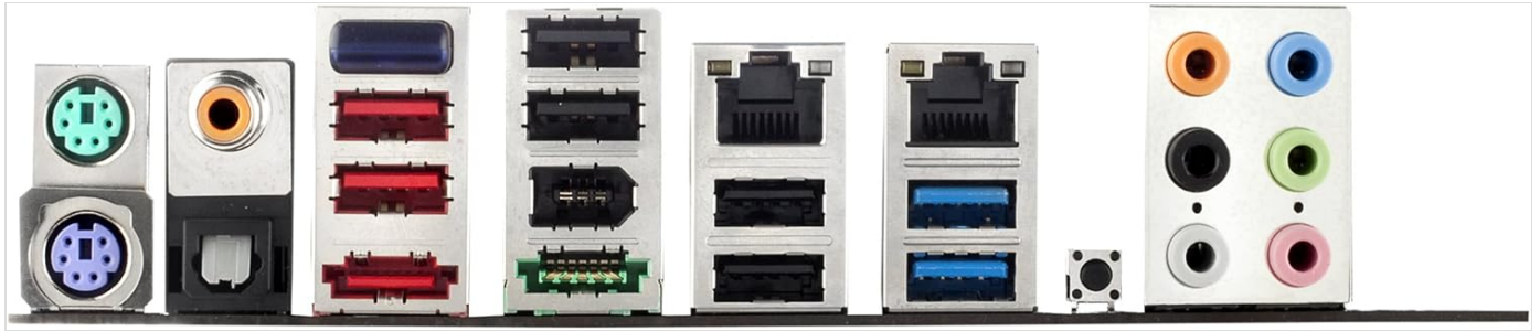
Figure 2.7.1: Rear I/O Panel of the ASUS P8P67 EVO motherboard.
