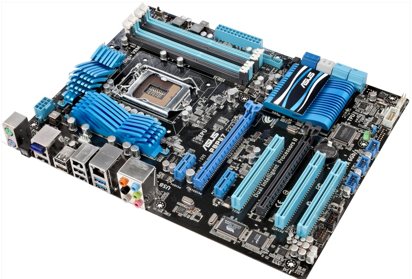
Figure 2.1: Top-down view of the ASUS P8P67 LE motherboard, highlighting major components such as the CPU socket, RAM slots, PCIe slots, and various headers.
