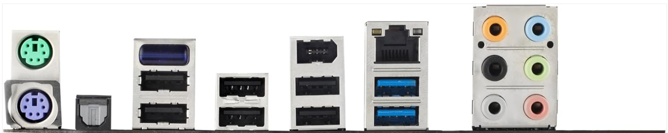
Figure 2.3: Rear I/O panel of the ASUS P8P67 LE motherboard, showing ports for USB 2.0, USB 3.0, LAN, audio, and PS/2 for keyboard/mouse.
