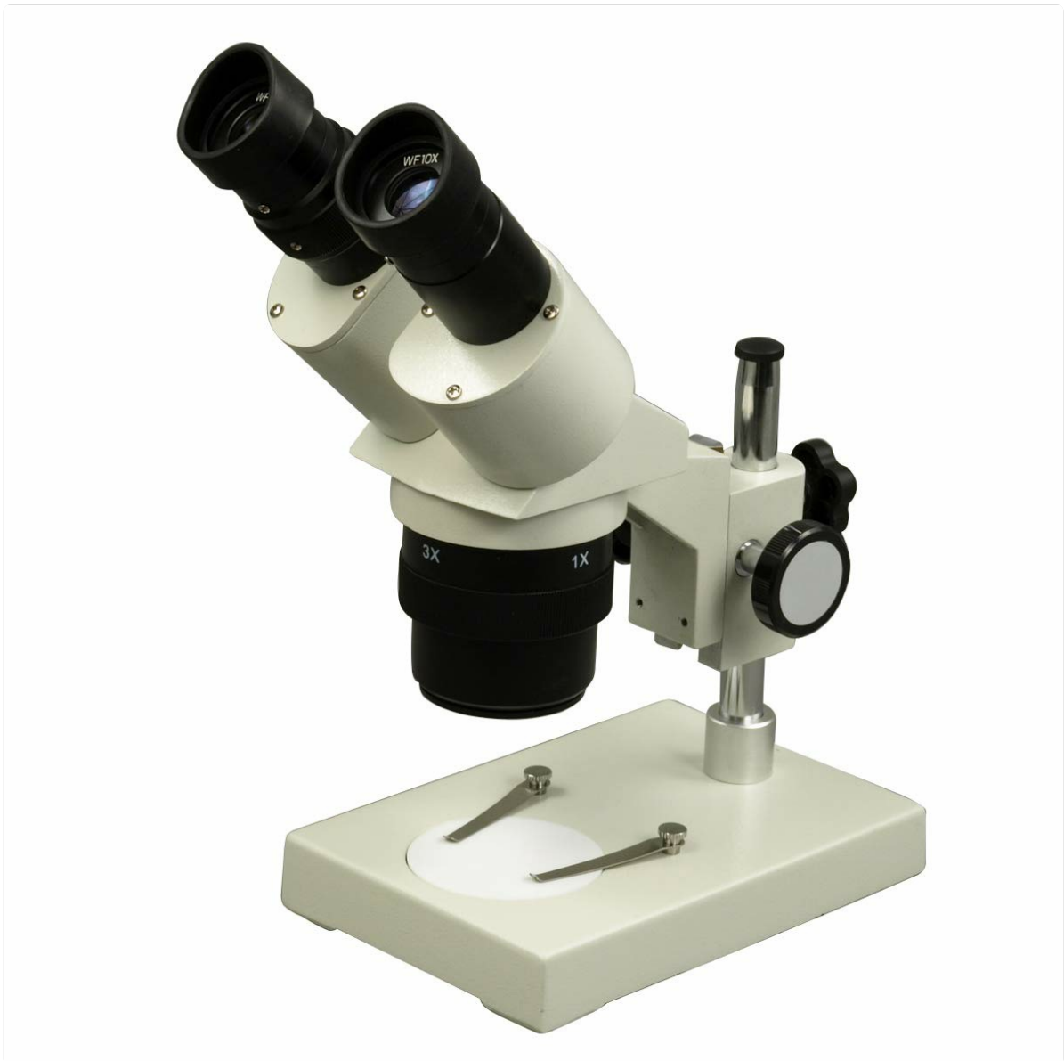
Figure 6: Objective turret for magnification selection.
