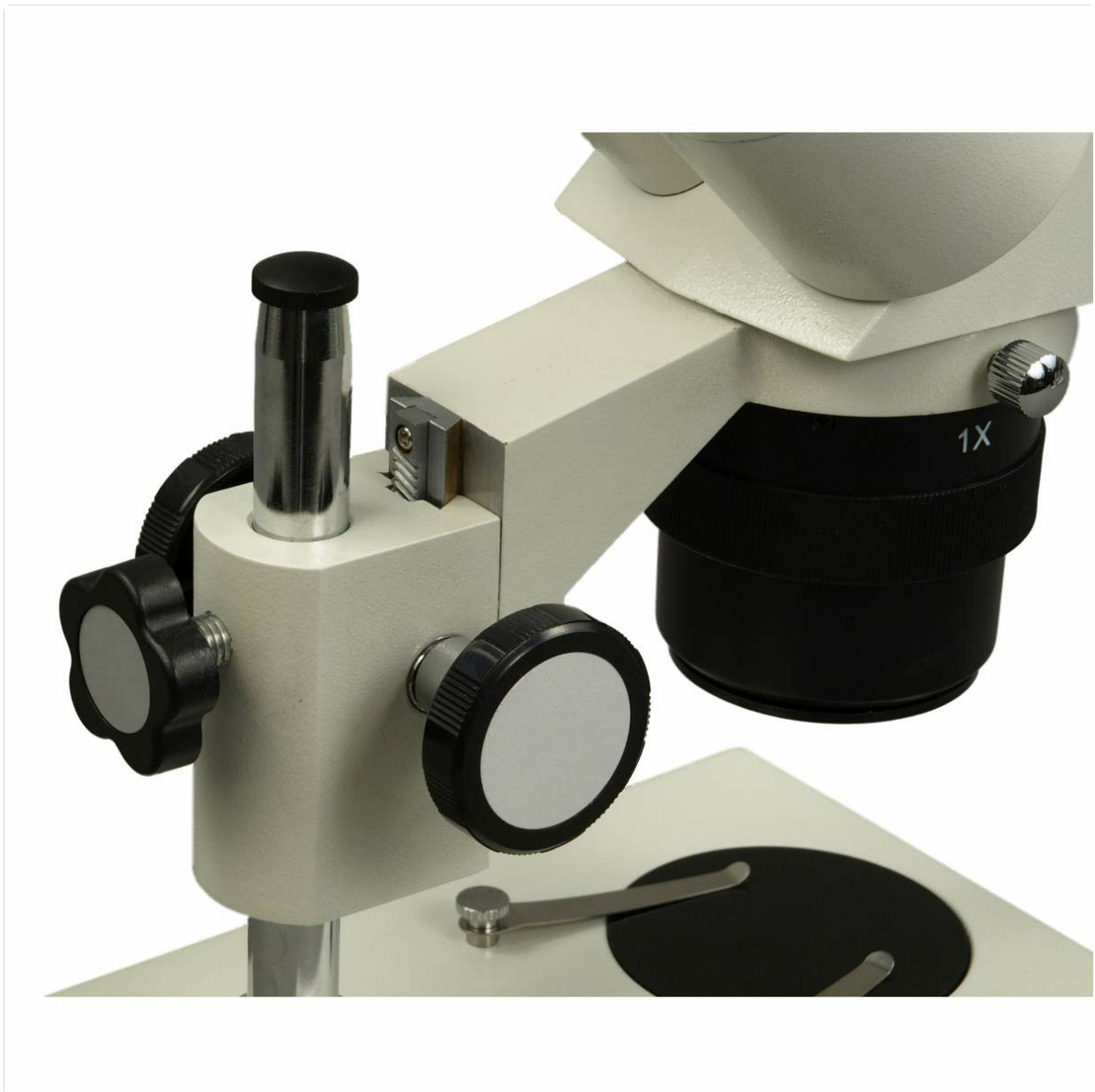
Figure 7: Coarse focus knob for adjusting image clarity.
