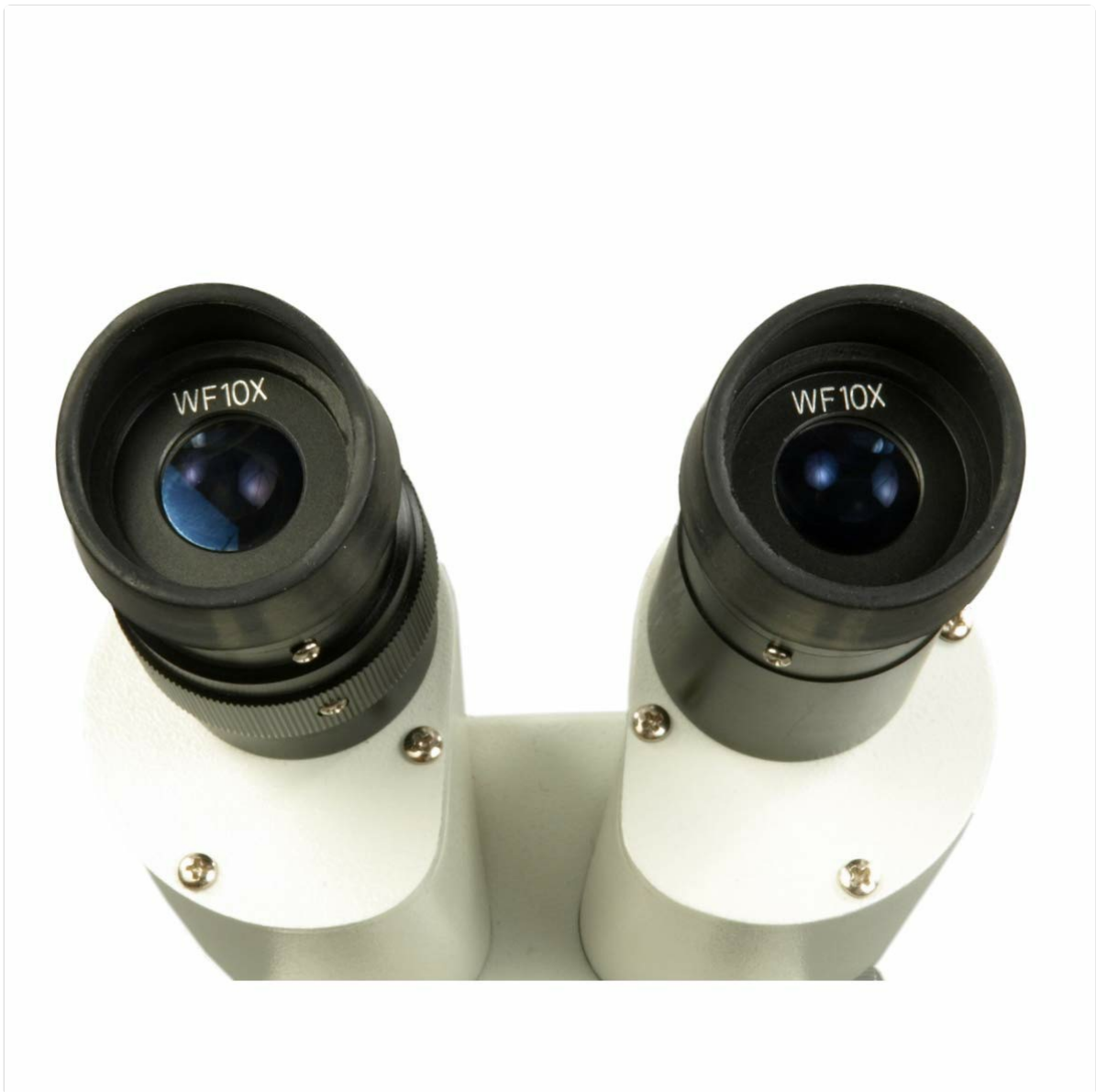
Figure 3: WF10X eyepieces in place.
