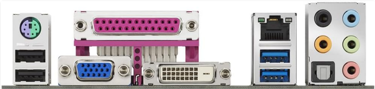
Figure 5: Close-up view of the rear I/O panel of the Intel DH61BE Motherboard, showing various ports including USB, Ethernet, audio, and video outputs.
