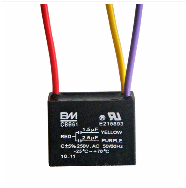
Image 1: BM CBB61 Ceiling Fan Capacitor. This image displays the capacitor unit with its three color-coded wires (Red, Yellow, Purple) and printed specifications including capacitance values (1.5µF, 2.5µF) and voltage (250V AC). The red wire is typically the common connection, while yellow and purple correspond to the specific capacitance values for fan speed control.
