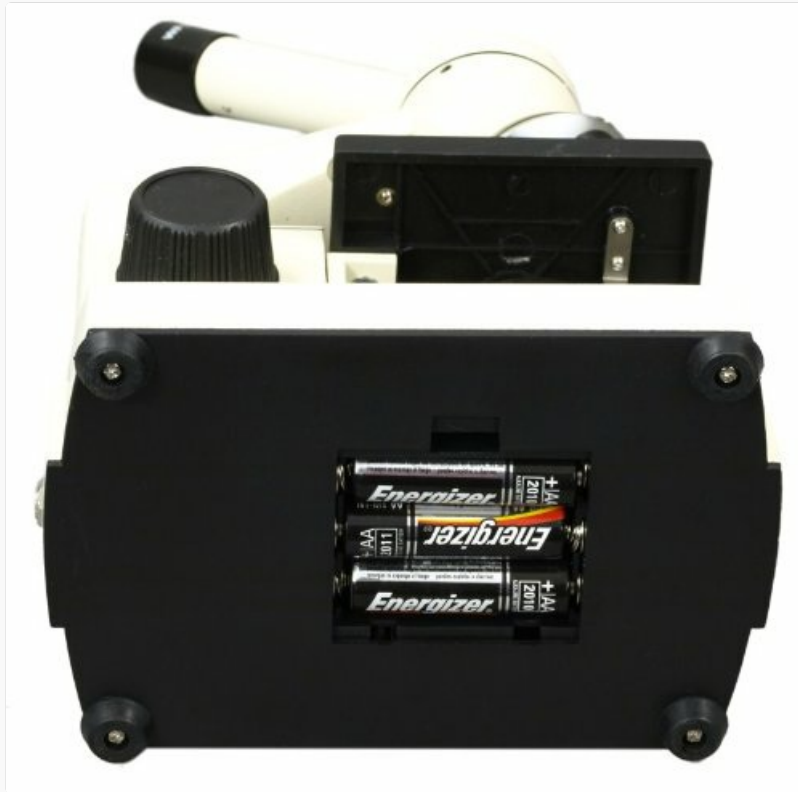
Figure 2.3: The underside of the microscope, illustrating the battery compartment designed to hold three AA batteries for portable operation.
