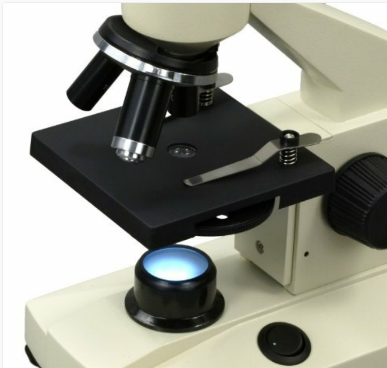
Figure 2.2: A close-up view of the microscope's stage and the integrated LED illumination system, highlighting the objective lenses and the disc diaphragm below the stage.
