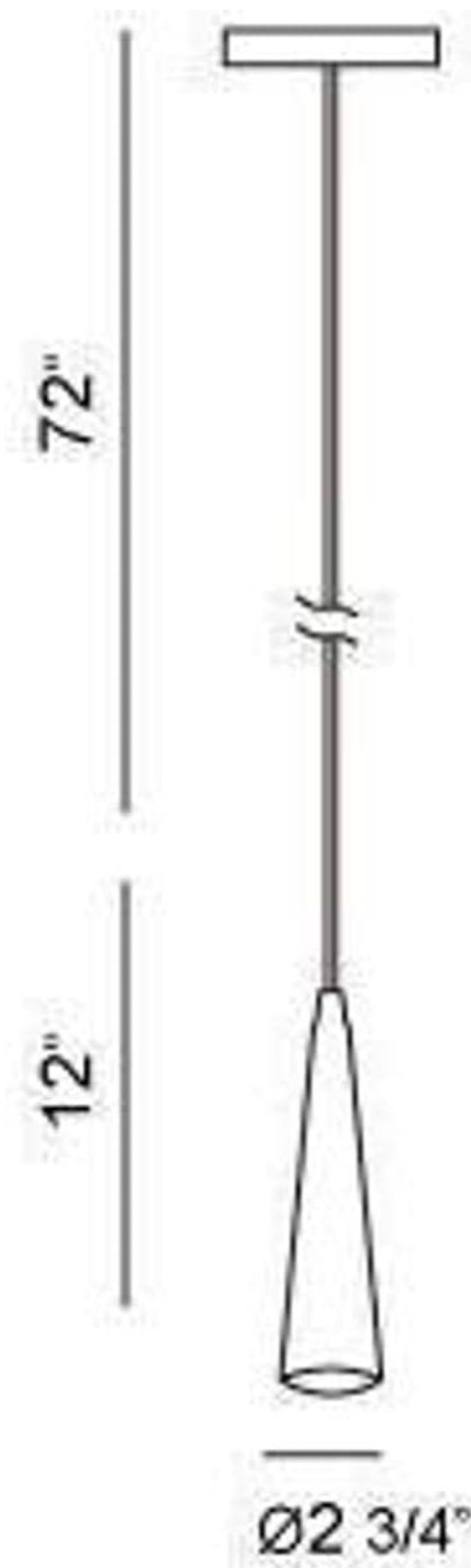
Image 4.1: Dimensional diagram of the pendant light, showing a 12-inch fixture length and a total adjustable cable length of up to 72 inches.
