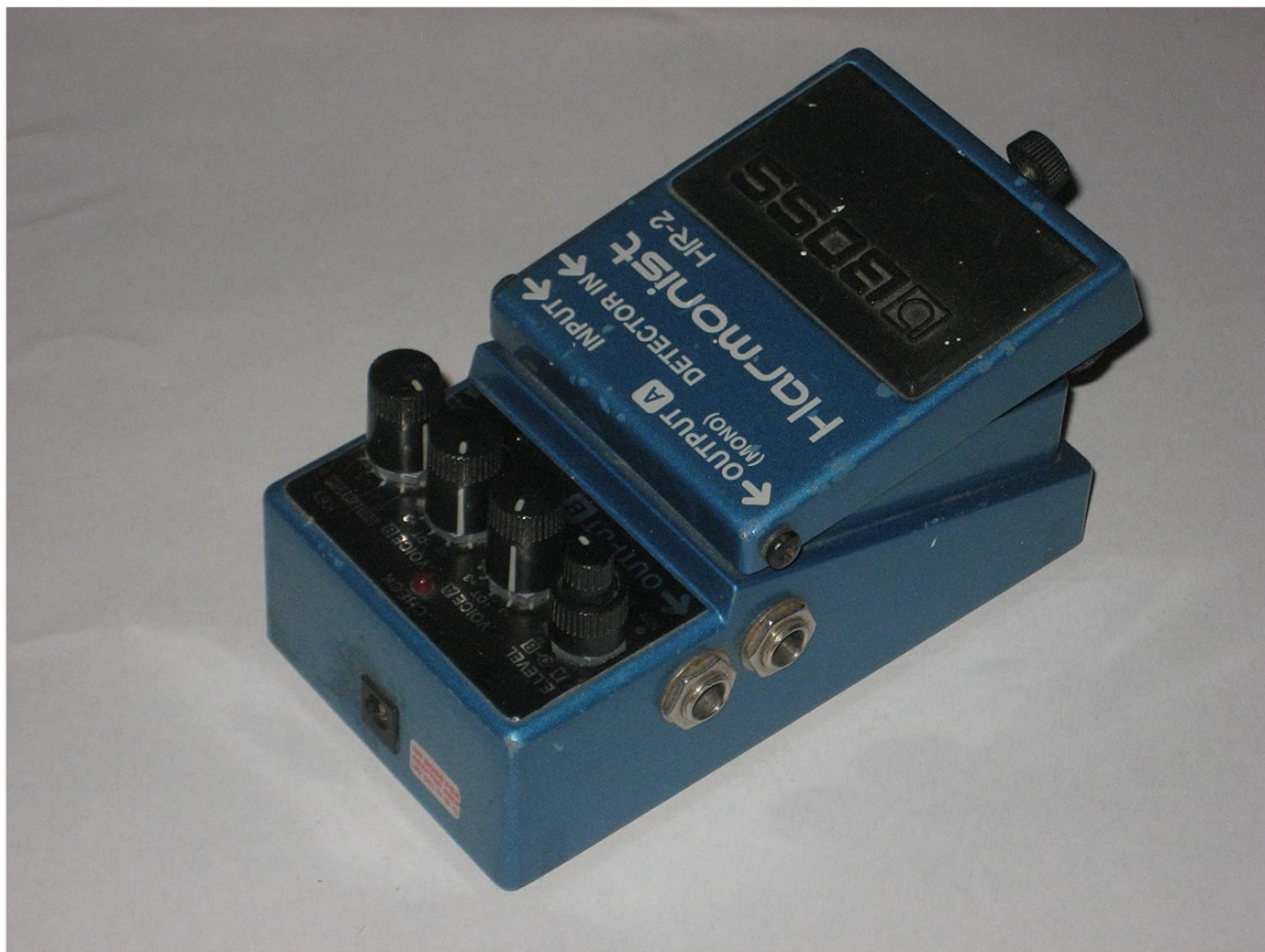
Figure 4: Side view of the HR-2 pedal, highlighting the input, output, and detector jacks.
