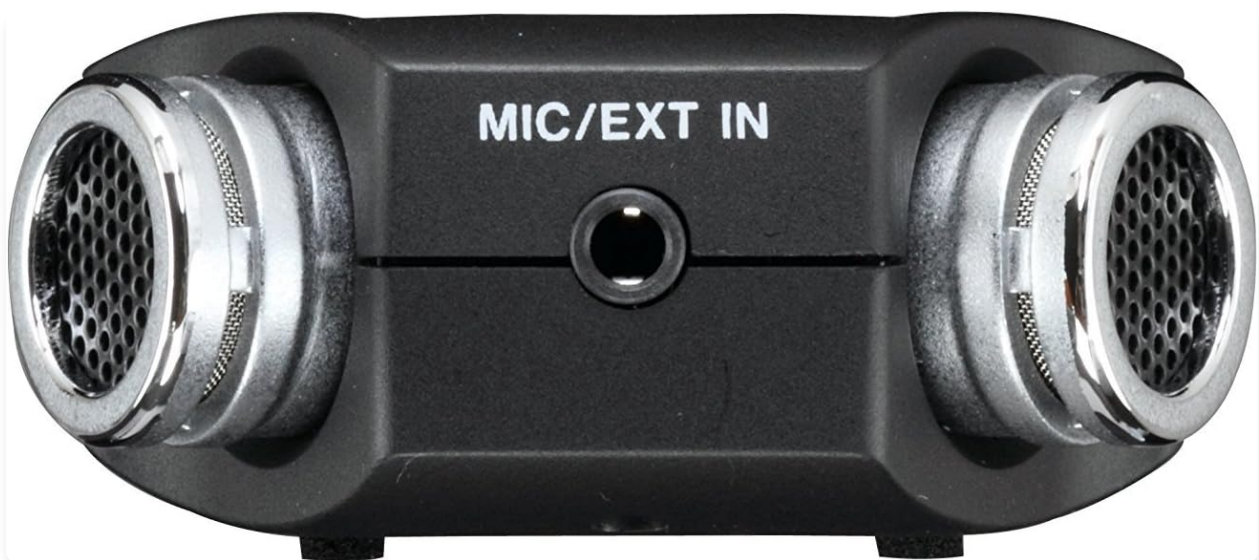
Figure 5: Top view of the DR-05 with built-in microphones and MIC/EXT IN port.
