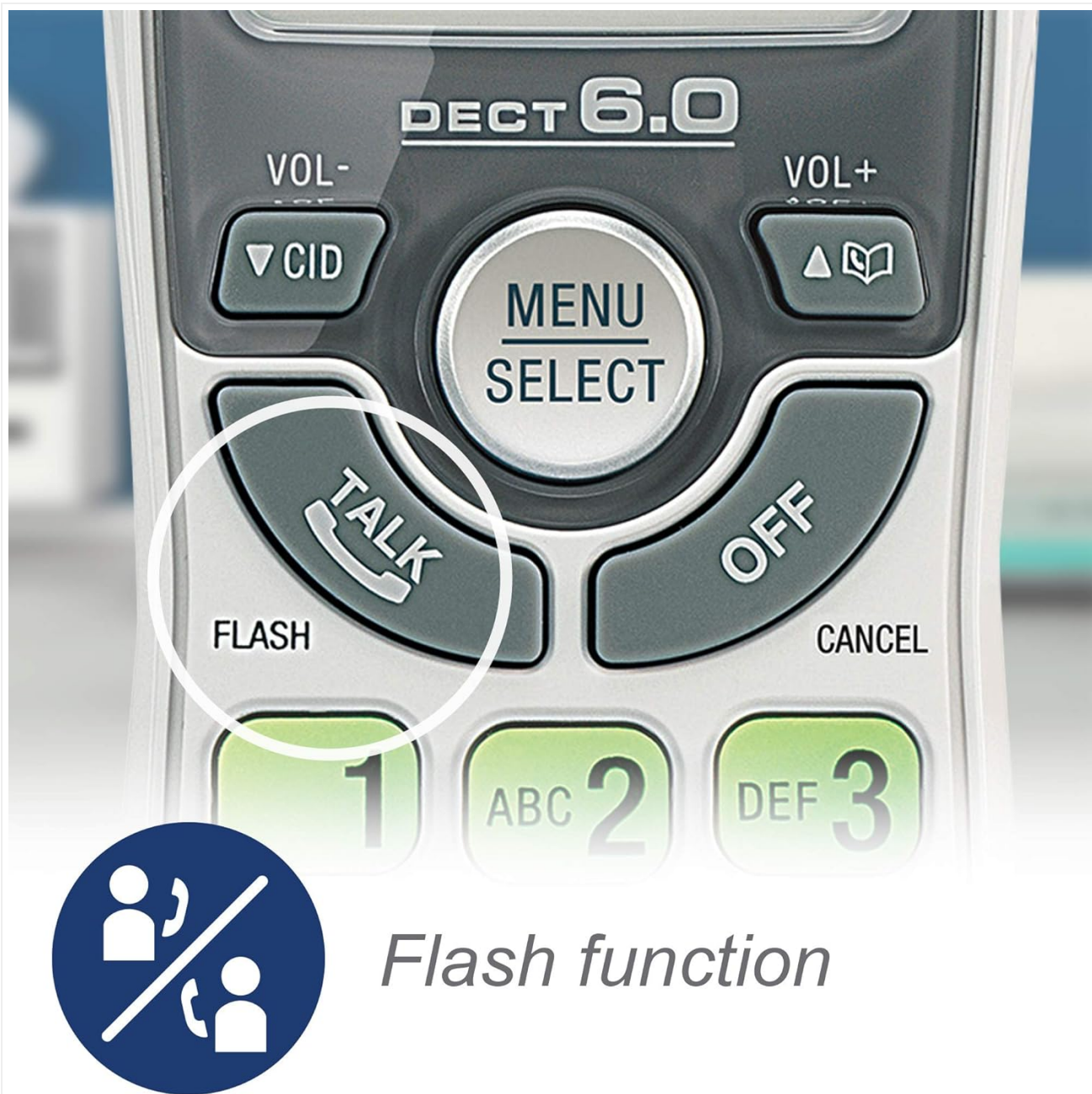
Figure 3: The Flash button on the handset allows for call waiting and other network features.
