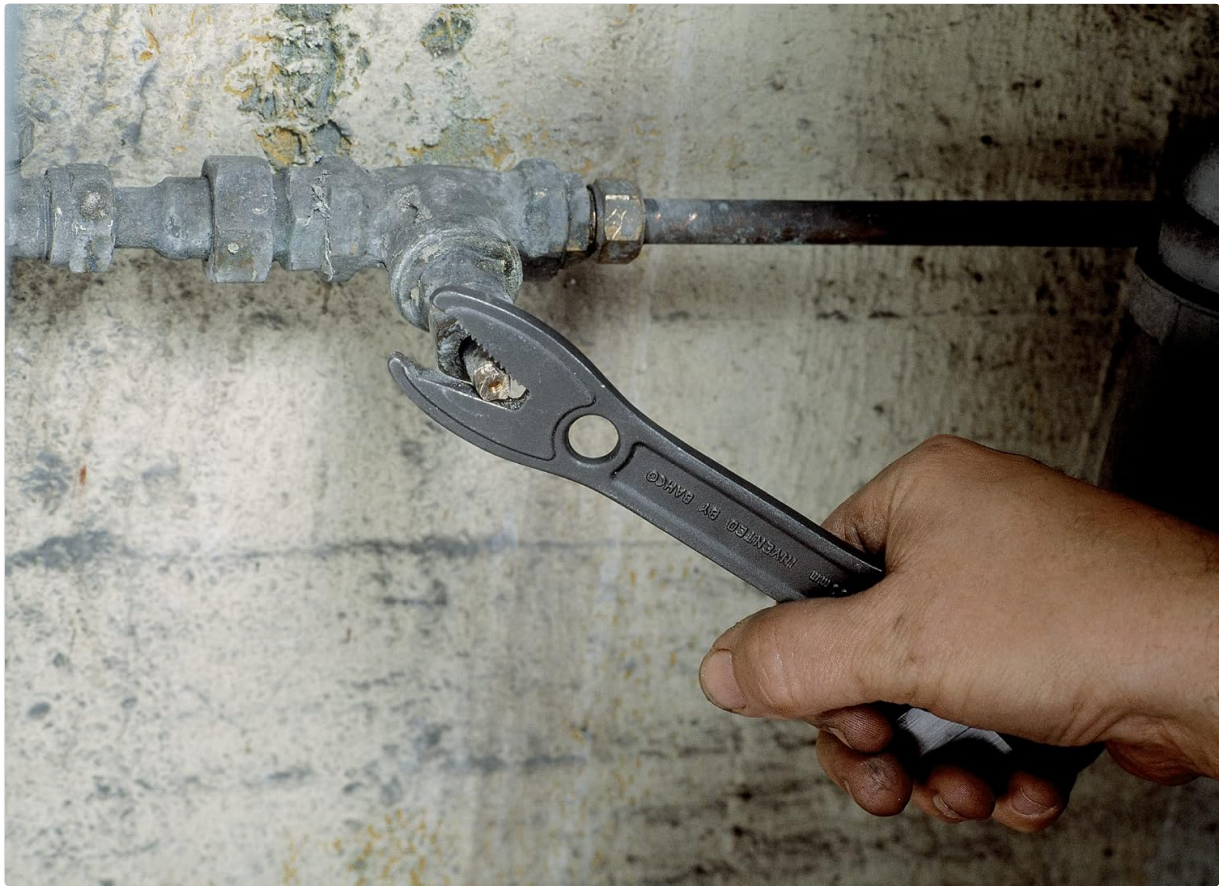
Figure 3: V-Jaw (Alligator Jaw) in Use. This image illustrates a hand utilizing the V-jaw end of the wrench to grip and turn a rounded pipe or fastener.
