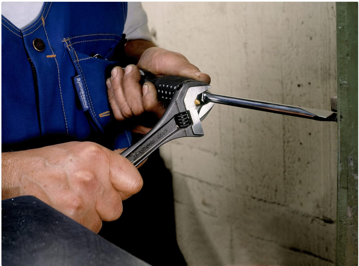
Figure 4: Wrench Used for Prying. This image shows the wrench being used to pry, demonstrating a potential secondary application.
