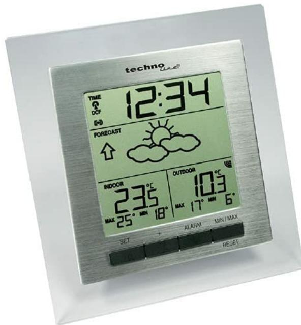
This image shows the Technoline WS 9136-IT Weather Station. The display features the current time (12:34), a DCF signal indicator, a weather forecast icon (partly cloudy), indoor temperature (23.5°C) with max/min values (25°C/18°C), and outdoor temperature (10.3°C) with max/min values (17°C/6°C). Buttons for 'SET', 'ALARM', 'MIN/MAX', and 'RESET' are visible below the display.
