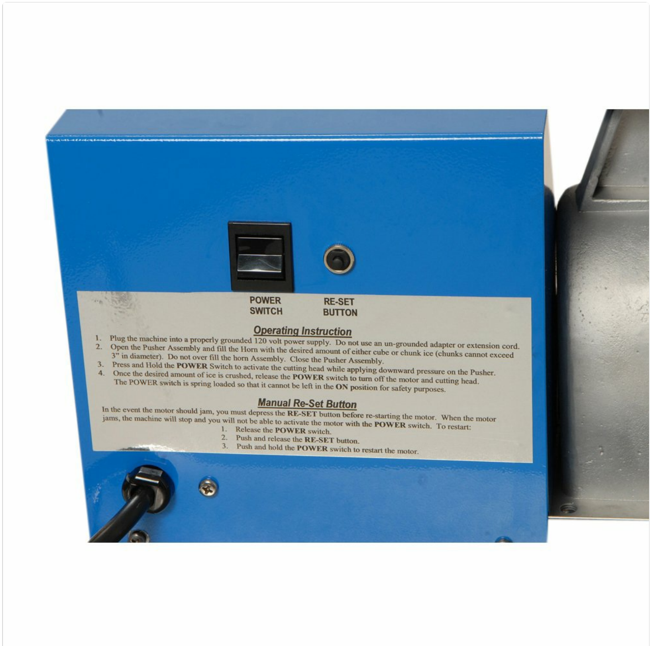
Figure 3: Control panel showing the POWER switch and RE-SET button, essential for operating and resetting the machine.
