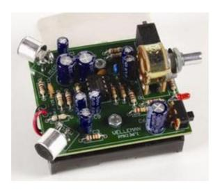
Image 1: Fully assembled Velleman MK136 Super Stereo Ear circuit board. This image shows the compact green PCB populated with various electronic components including resistors, capacitors, integrated circuits, two electret microphones (one on each side), a volume potentiometer, and a headphone jack. The board is designed for a 9V battery power source.
