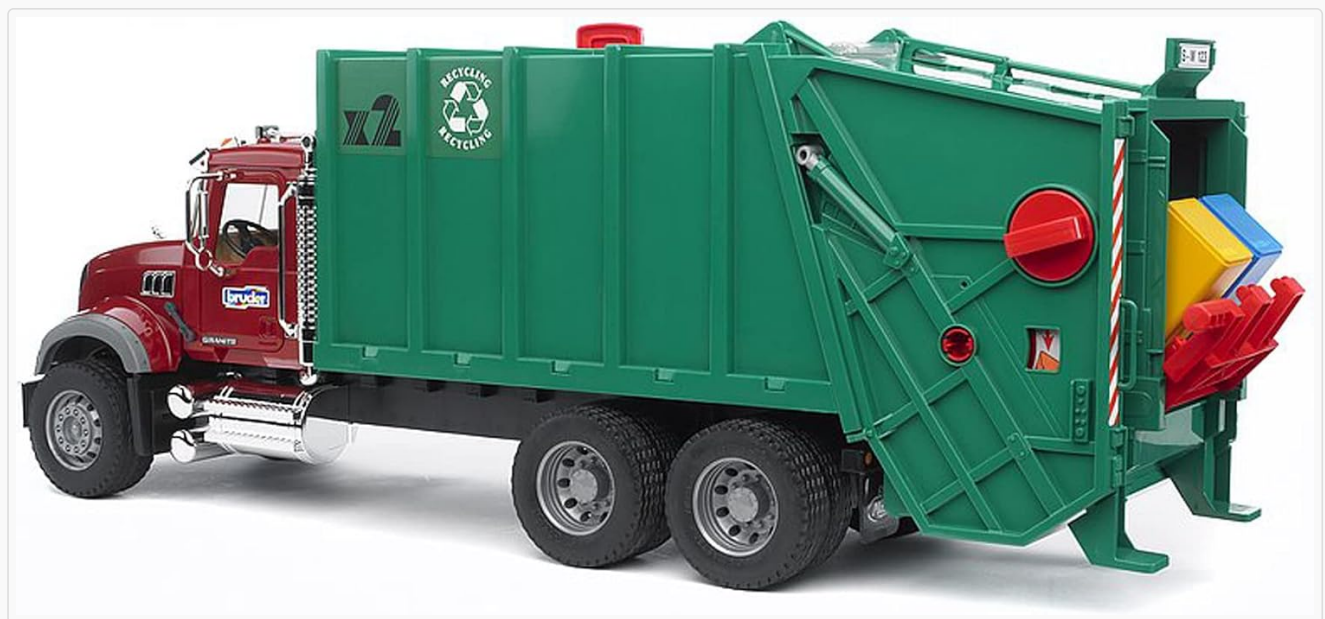
Figure 3: Rear view showing the dustbin lift in action.
