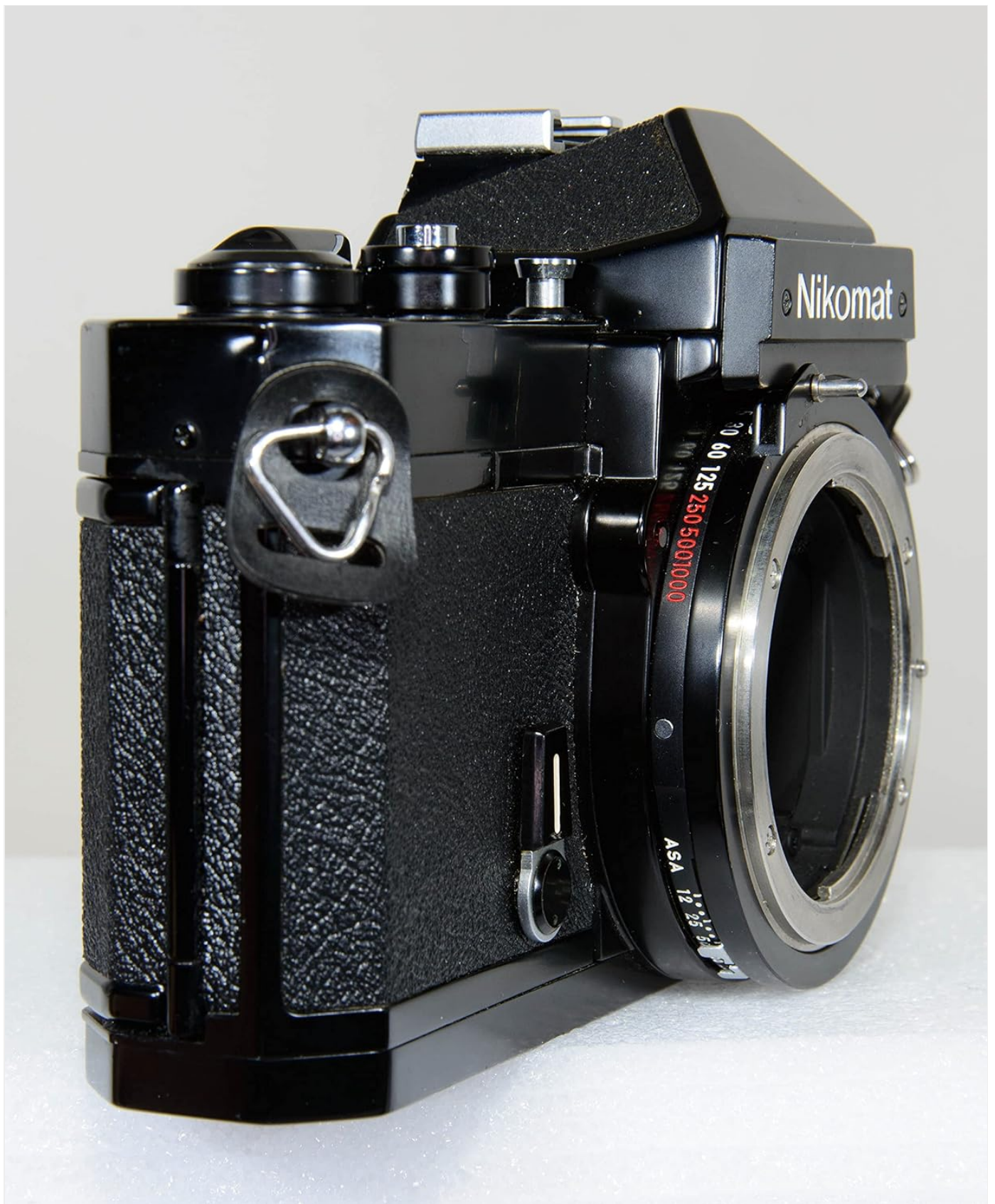
Figure 6: Another angled side view of the Nikkormat FT2, showing the self-timer lever and depth-of-field preview button near the lens mount.
