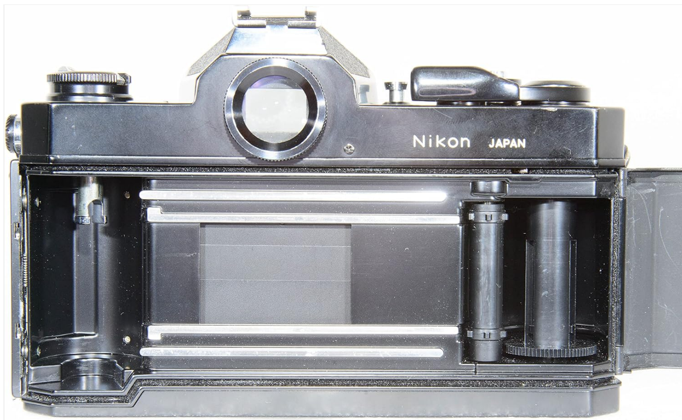
Figure 7: Internal view of the Nikkormat FT2 film compartment with the back open, revealing the film pressure plate, film rails, and take-up spool.
