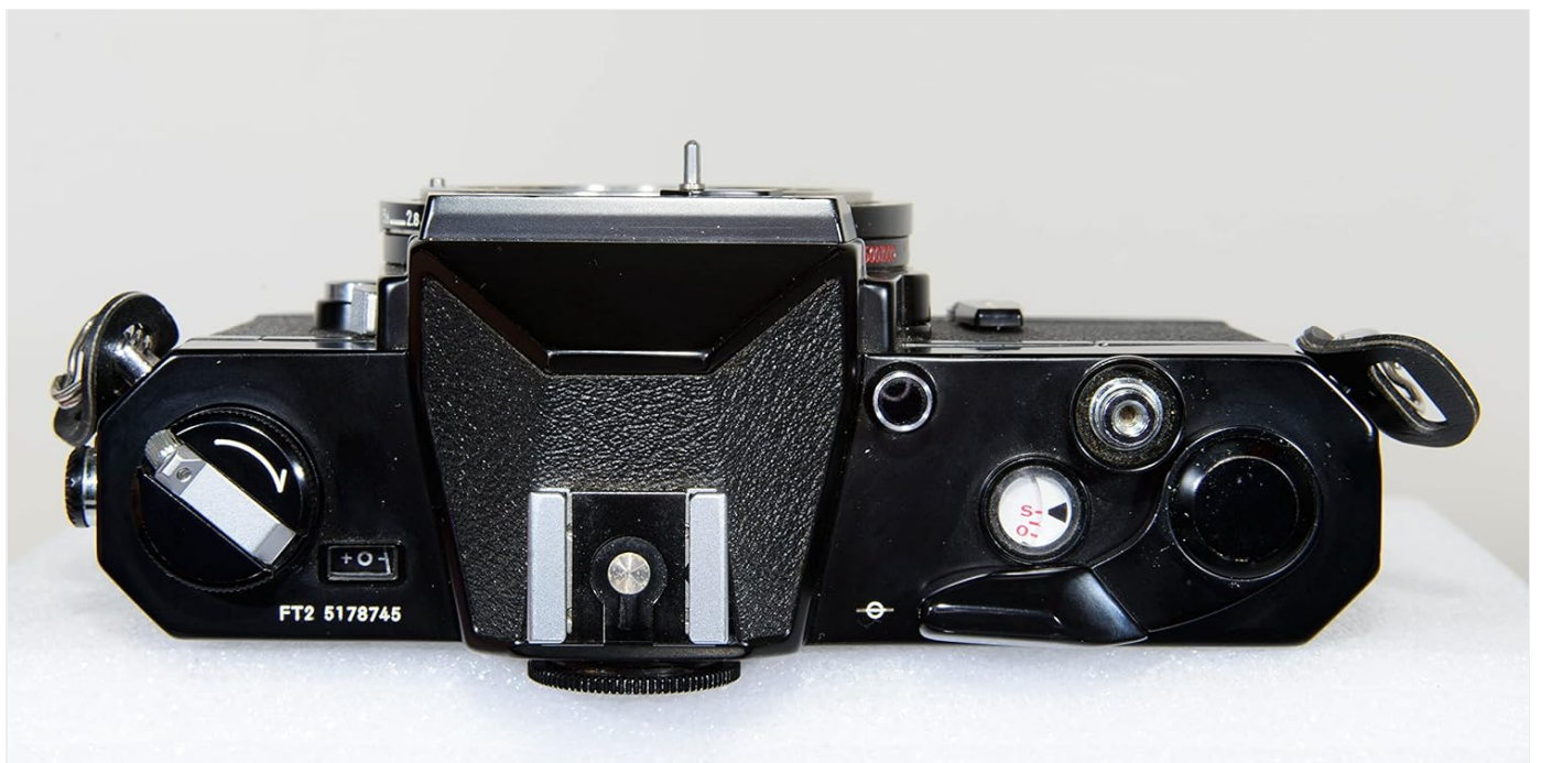
Figure 3: Top view of the Nikkormat FT2, featuring the shutter speed dial, film counter, film advance lever, shutter release button, and the hot shoe for flash synchronization.
