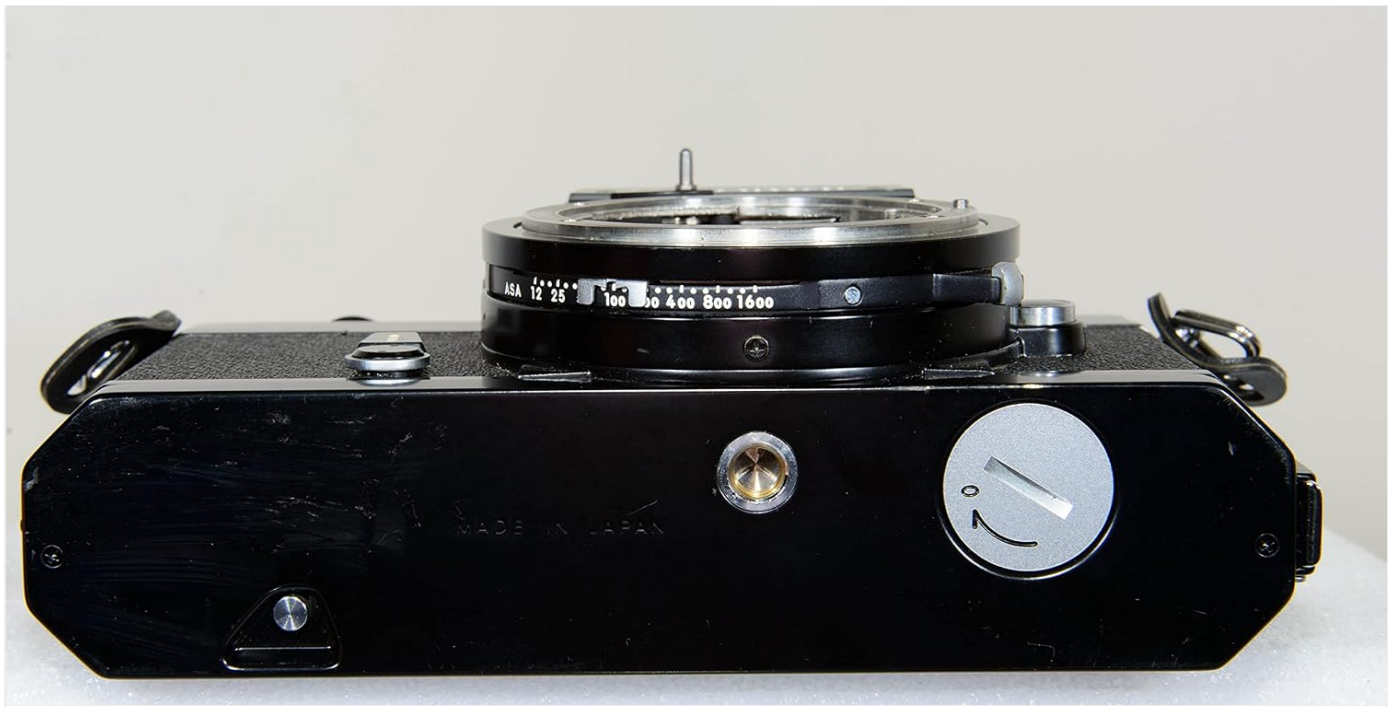
Figure 4: Bottom view of the Nikkormat FT2, illustrating the battery compartment cover and the standard tripod mounting socket.
