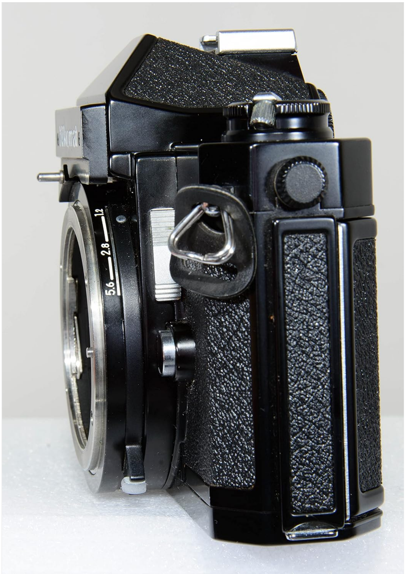
Figure 5: Angled side view of the Nikkormat FT2, displaying the film rewind crank and a strap lug.
