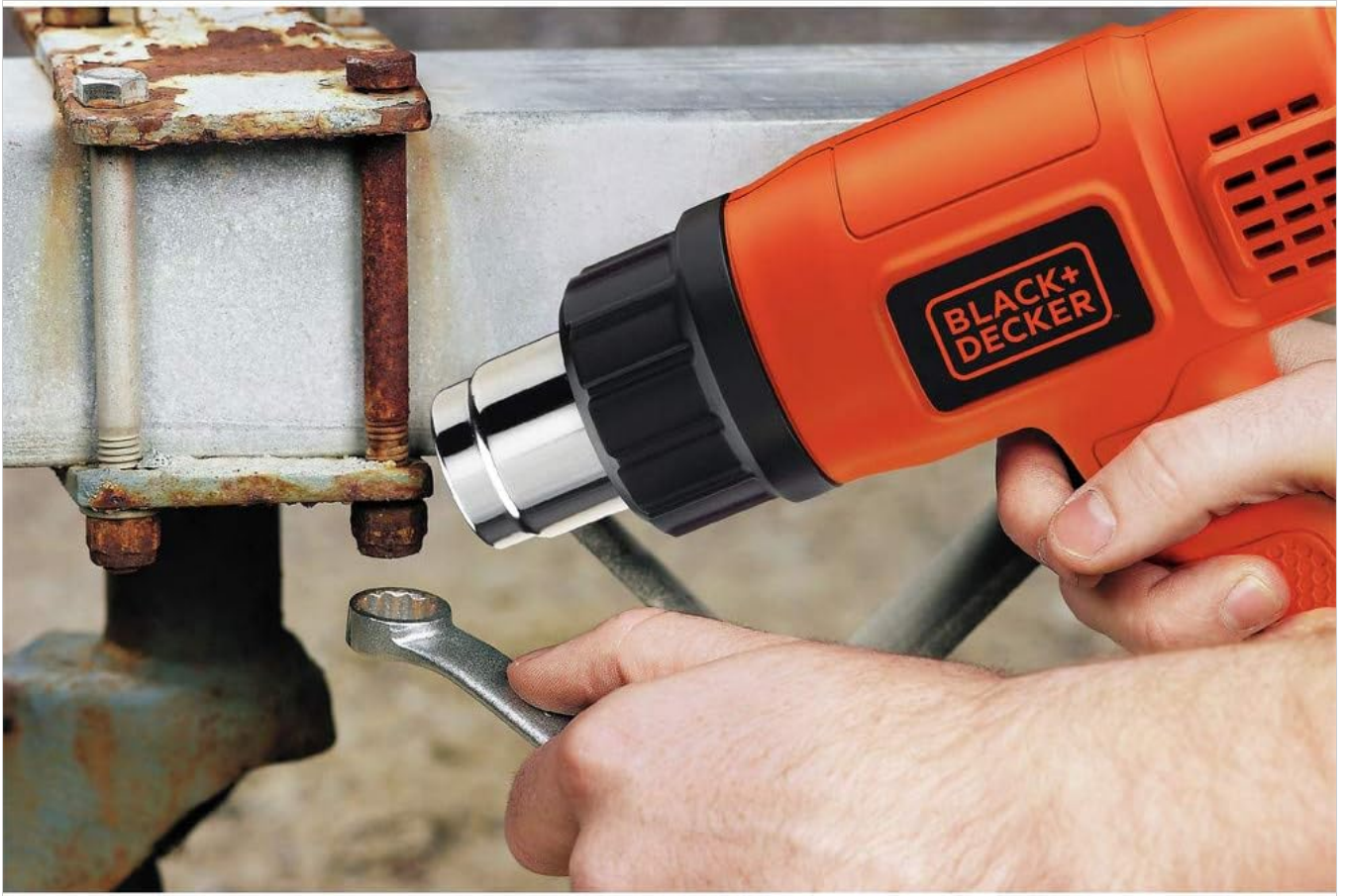
Figure 5: Applying heat to loosen a rusted bolt.
