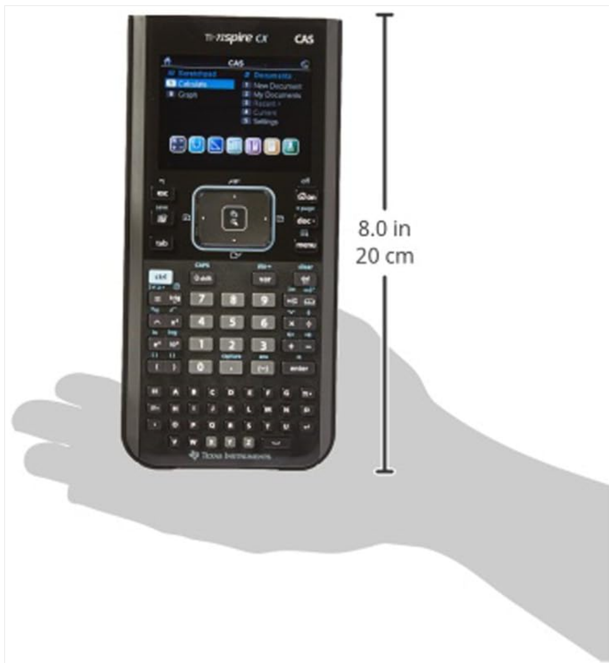
Figure 7.1: The TI-Nspire CX CAS calculator held in a hand, illustrating its physical dimensions. The image shows the calculator is approximately 8.0 inches (20 cm) in length, providing a visual reference for its size.
