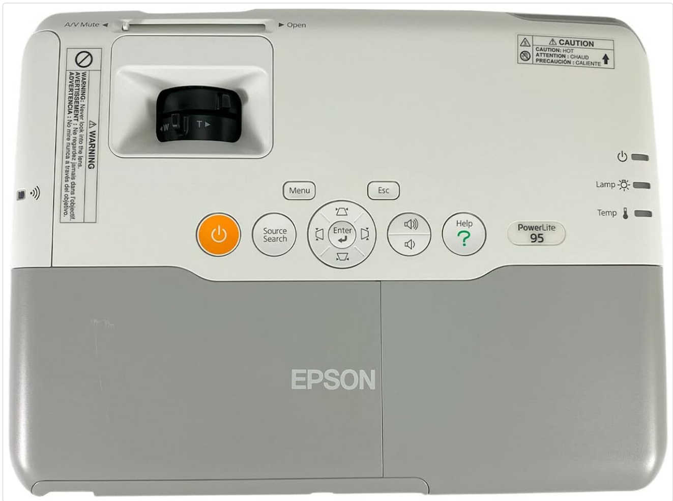
Figure 2.2: Top panel of the Epson PowerLite 95 Projector, displaying power button, menu, source search, and navigation controls.
