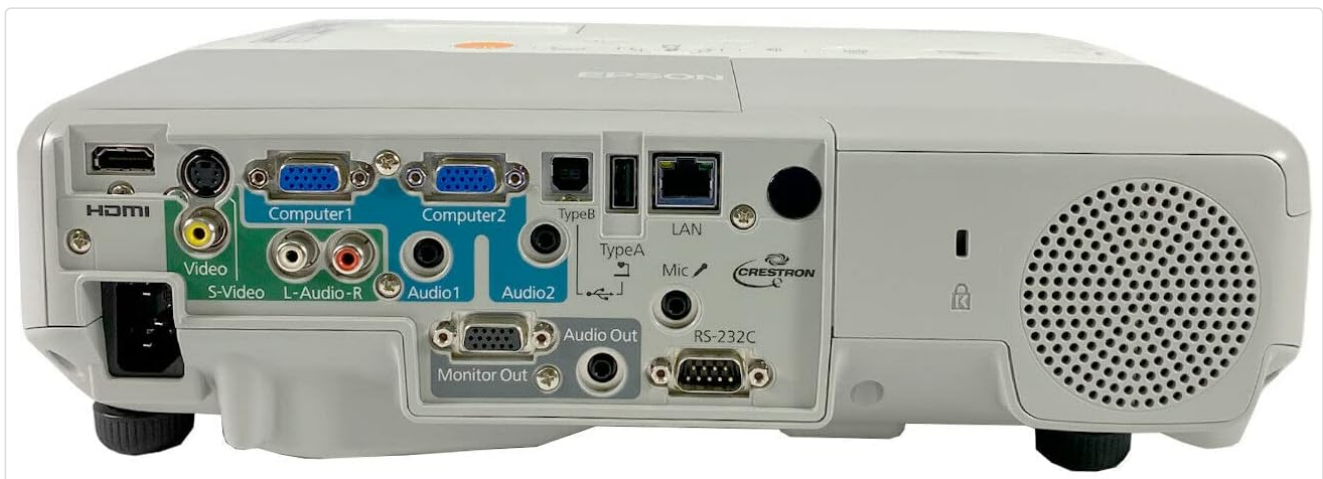
Figure 2.3: Rear panel of the Epson PowerLite 95 Projector, showing HDMI, Video, S-Video, Audio, Computer (VGA), Monitor Out, LAN, USB (Type A and B), and RS-232C ports.
