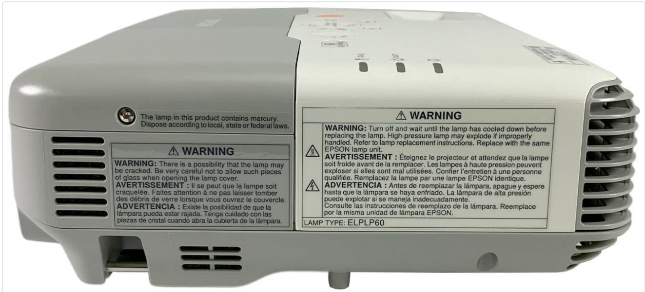
Figure 5.1: Side view of the projector showing a warning label regarding lamp replacement. Always turn off and wait for the lamp to cool down before replacing.
