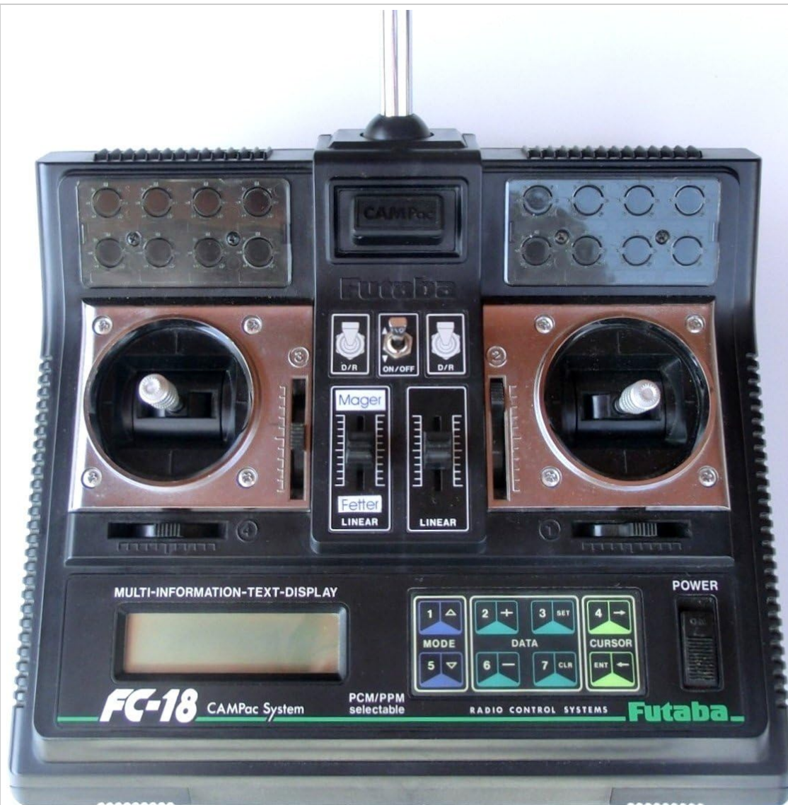
Figure 3.1: Futaba FC-18 35 MHz Transmitter Front View
