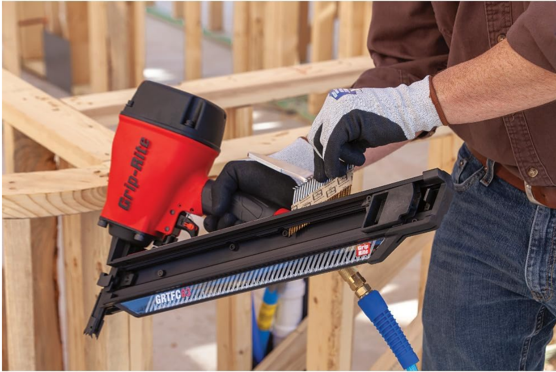
Figure 3.1: Demonstrates the proper method for loading a strip of paper tape framing nails into the tool's magazine.
