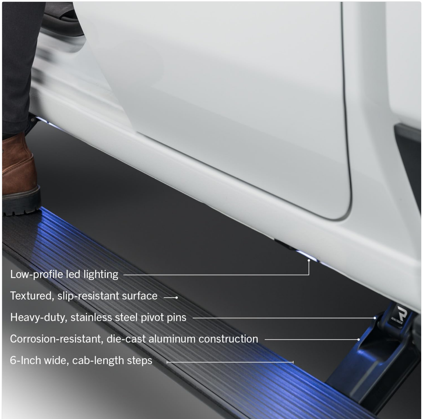
Image: Detailed view highlighting the key features of the PowerStep, including LED lights and durable construction.
