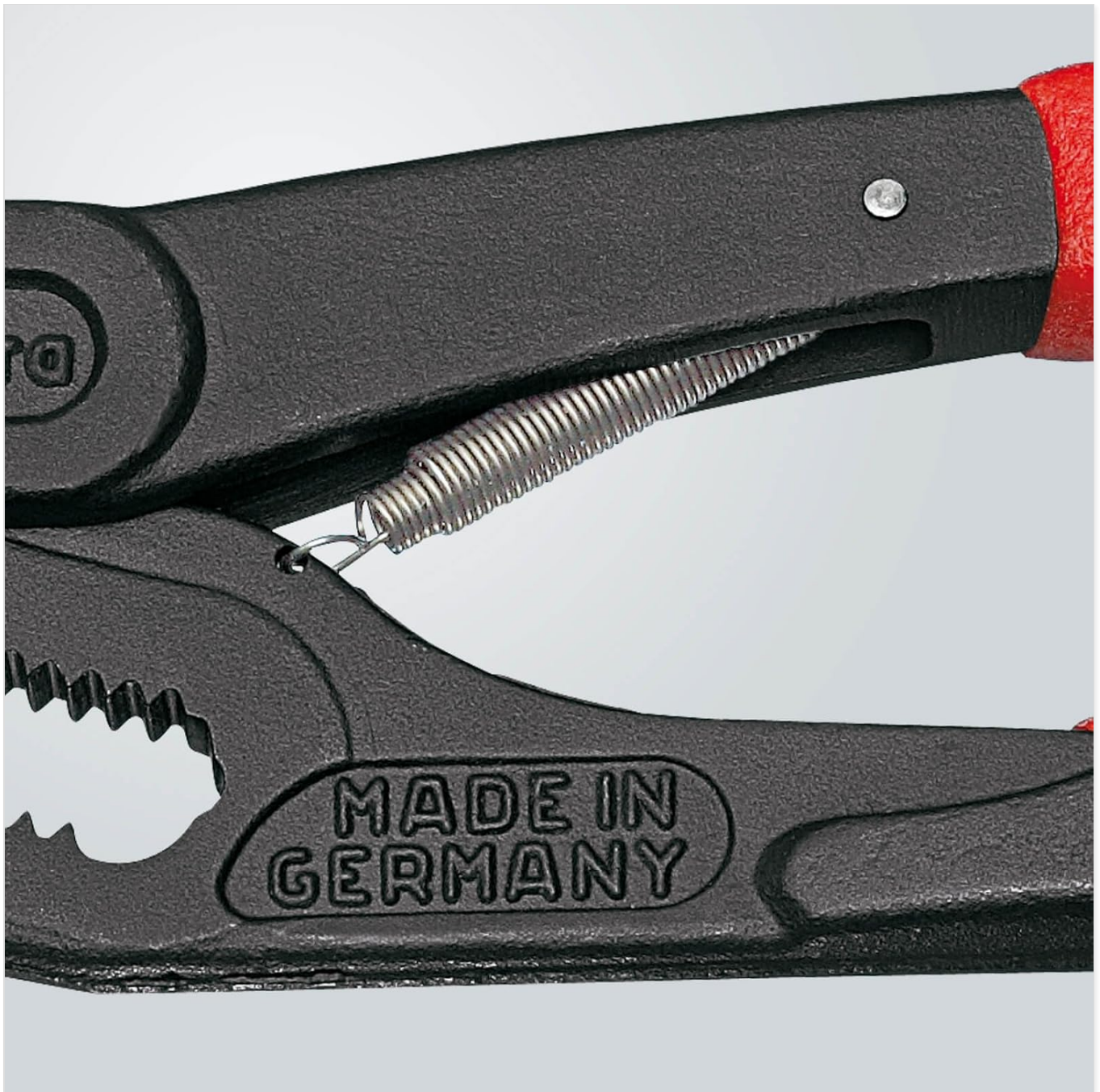
Image 3.2: View of the internal sheltered spring, which facilitates the automatic closing and adjustment of the pliers.
