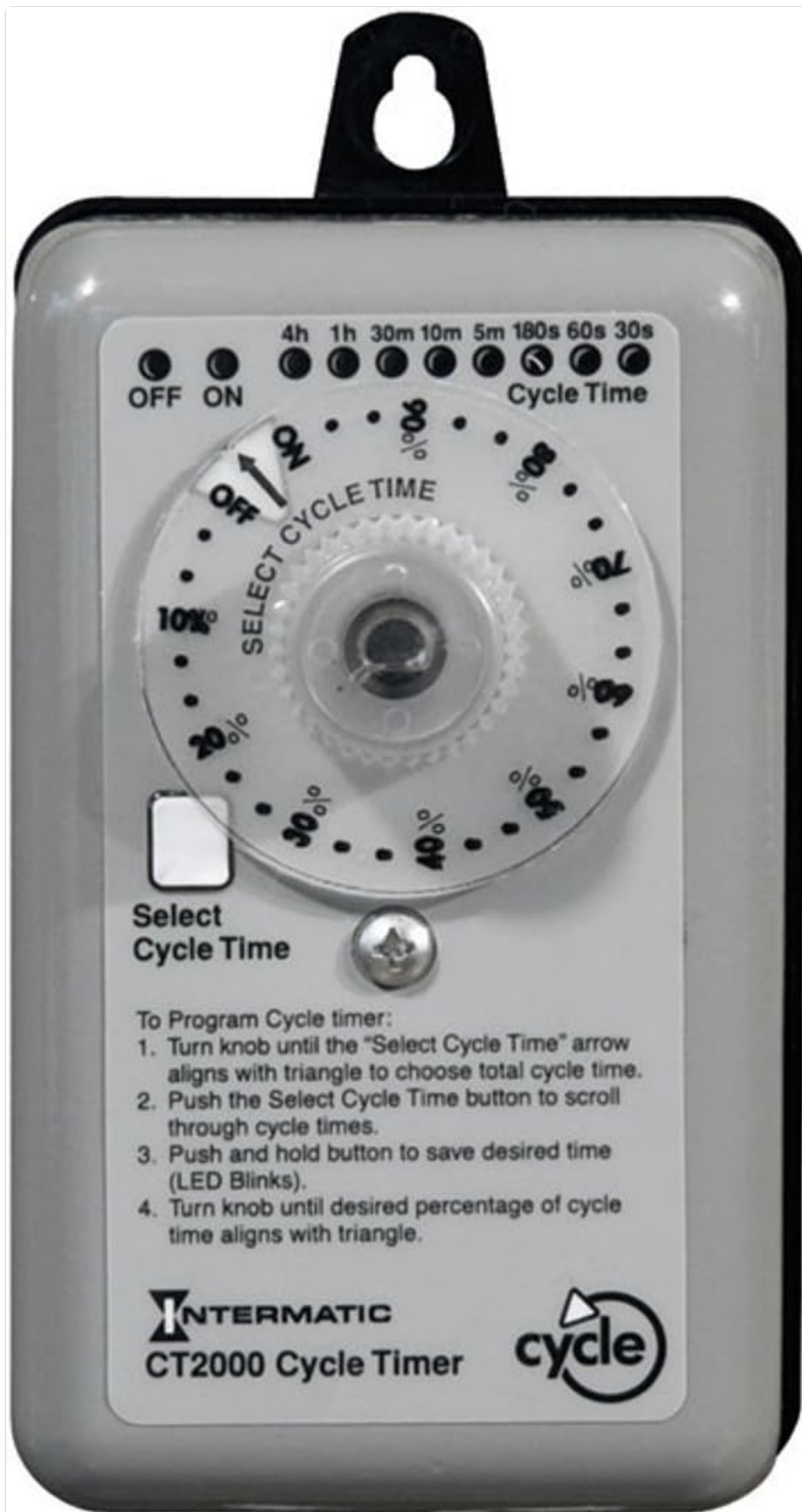
Figure 1: Front view of the Intermatic CT2000 Percentage Cycle Time Switch. The image displays the main dial for percentage ON time selection, the 'Select Cycle Time' button, and a row of LEDs indicating the chosen cycle duration (30s, 60s, 180s, 5m, 10m, 30m, 1h, 4h). Instructions for programming the cycle timer are printed on the lower part of the device's label.
