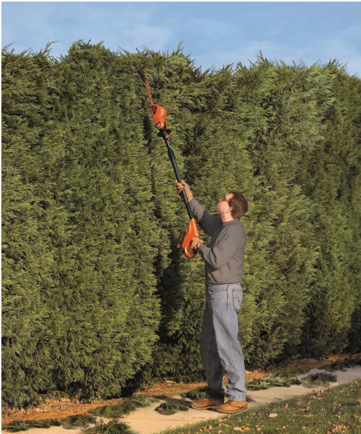
Figure 5: A user demonstrating the extended reach of the pole hedge trimmer to trim the top of a tall hedge.
