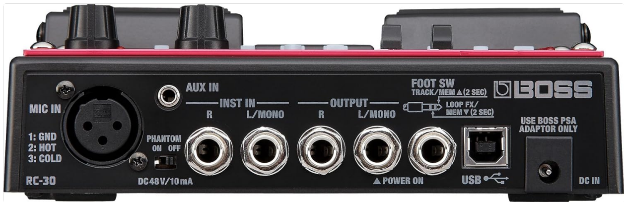
Image: Rear view of the BOSS RC-30, showing the MIC IN (XLR), AUX IN, INST IN (L/MONO, R), OUTPUT (L/MONO, R), FOOT SW, USB, and DC IN ports.
