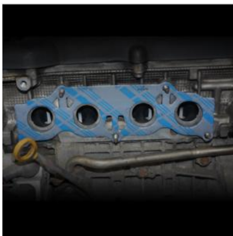
Figure 5: An exhaust manifold gasket correctly installed on an engine, demonstrating its position between the cylinder head and manifold.
